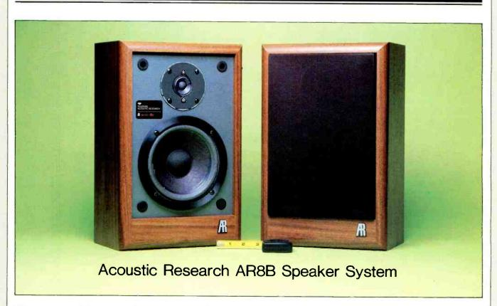
THE two-way AR8B is the smallest and least expensive speaker system in the current Acoustic Research line. Like all AR speakers, it is an acoustic-suspension model, and it has a newly designed 6-inch woofer that crosses over at 2,000 Hz to a 11/4-inch "liquid cooled" cone tweeter. (The tweeter
