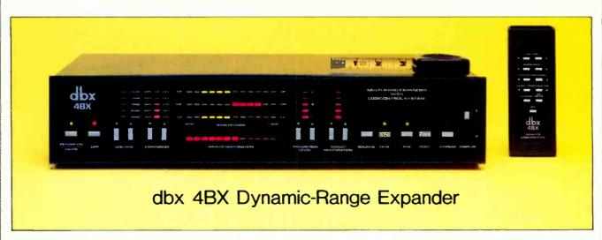
THE dbx Model 4BX three-band dynamic-range expander features an "impact restoration" circuit and a wireless (infrared) remote control that duplicates all of its expansion controls and most of the frontpanel function switches. The 4BX is normally connected to the tape input and output jacks of the system amplifier, and it duplicates their functions on its rear apron. It also has front-panel controls to expand a signal either before it is recorded or after it
