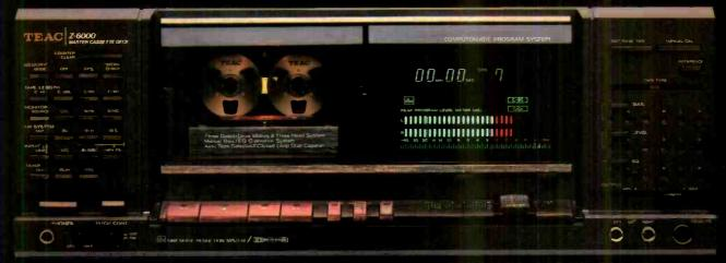
3 Heads (Ferrite Play, Sendust Rec), 3 Motors, Direct Drive Capstan Motor, Dual Capstan, dbx, Dolby B & C NR, dbx Disc Position, Manual & Reference Bias/
