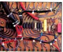
The quality of workmanship that goes into building a Mark Levinson ML-3 was apparent the moment we took the covers off. The two large black toriodal transformers and four 36,000-µF capacitors dominate the interior. The bottom photo shows a close-up of the output-amplifier circuit board.
