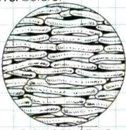
PACKING DENSITY OF UNIFORM PARTICLES.
