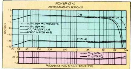
The upper curves indicate overall record-playback response at the manufacturer's indicated 0-dB recording level using the tapes designated on the graph. In the center are the same measurements recorded at -20 dB relative to the upper curves, a level used for frequency-response measurements. Bottom curves show playback response with calibrated test tapes and indicate performance with prerecorded tapes.
