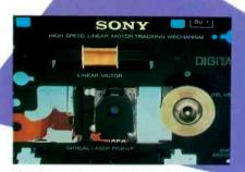
SONY'S CD PLAYER REFINEMENTS INCLUDED UNILINEAR" CLOCK CIRCUITRY, PLUS THE FIRST 8X OVERSAMPLING FILTER AND 18-BIT CONVERTERS. WE ALSO CREATED DIGITAL SYNC" CIRCUITRY, ONE-BIT PULSE CONVERTERS, AND THE LINEAR MOTOR LASER TRANSPORT SHOWN. THE TRANSPORT WAS THE FIRST TO CUT TRACK ACCESS TIME TO UNDER ONE SECOND.
