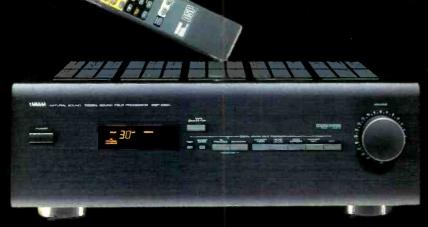
Yamaha's DSP-E200 (S499) offers a digital Dolby Pro Logic decoder, a four-mode ambience processor, and three 25-watt amplifiers to power one center and two surrounc speakers. A full-function wireless remote control is included.
