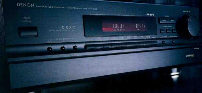
Just as discrete components allow an audio system to be optimized for better sound, Denon's DDSC produces more accurate, more realistic surround sound by reducing Total Harmonic Distortion, by increasing Signal-to-Noise and minimizing DSP quantization noise.
