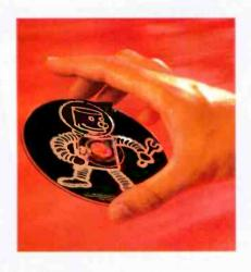
A CD player's laser can focus quite easily through a fingerprint, but excessive dirt or deep scratches can cause skipping and other audible glitches during playback. While there's a much greater margin of error than with a vinyl LP, it just makes sense to keep your oily fingers off the playing surface (as well as the label side) by holding your CD's firmly at the rim as shown, or with your thumb or index finger anchored in the center.
