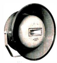
Weatherproof coaxial speaker; lowand high-frequency units enclosed in projection made of glass fibre with aluminum outer horn; 30 watts; 60 to 15,000 cps; 16-ohms impedance; 8" woofer and horn-loaded compression driver high-frequency unit; 2,000 cps crossover; 243%" diameter, 113%" deep.
