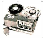
Portable; 3¾ and 7½ ips; monaural; frequency response ±3 db 40-8000 cps, at 7½ ips; takes 7" reels; wow and flutter less than 0.3%; distortion less than 0.8%; 2-level recording indicator; high-speed rewind lever; complete with ceramic mike; 10½" x 11¾ x 6½".
