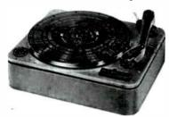
Four speeds; push-button operation; four-pole shock-mounted motor: balanced 4½-lb. turntable: plastic tone arm: intermixes 10" and 12" records; record repeat, stop, and pause features; scratch filter: jam-proof mechanism; plug-in heads accommodate monaural stereo cartridges: adjustable stylus pressure: 12½"x10½", clearance required 2½" above and 2¾" below.
