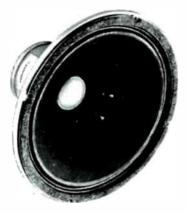
Wide range single cone unit with duralumin diaphragm to extend high frequency response: specially treated surround: 40 to 14,000 cps ±4 db: flux density 14,000 gauss: 20 ohms: 2" voice coil diameter: resonance at 40 cps; power rating 15 watts; depth 7"...\$79.00
