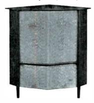
Frequency response from 30 to 22,000 cps; free of peaks, false bass, treble rise, or other frequency accentuations; system consists of two 15" 803A woofers, the 802D high frequency driver mounted on the 511B sectoral horn, and a 500 cps dividing network; bass reflex principle: 46½"h x 42½"w x 26½"d. In blond, walnut or mahogany.
