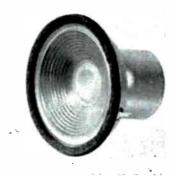
4" cone tweeter; capacity 10 watts; frequency response 2000 to 18,000 cps; 8 and 16 ohms impedance; 3 oz magnet; flux density 8000; baffle opening 33/8": wt 11/4 lbs ......\$12,50
