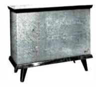
Mahogany, walnut or birch veneer infinite baffle enclosure; 35 to 16,000 cps; 3-way speaker system; 800 and 2,500 cps crossover frequencies; two B-207A coaxial speakers, one B-209 mid-range, one N-102 crossover network; handles 30 watts continuous, peaks to 60 watts: 16-ohms impedance; 36½"w x18½"d x32"h; 110 lbs.
