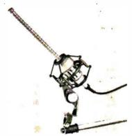
Dynamic directional; can be used with boom; frequency response 30–10.000 cps; impedance 50, 150, 250 ohms; output –48 db; length 17% x3%6.
