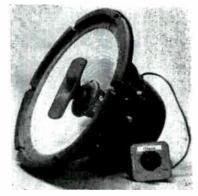
12" coaxial speaker with tweeter level control and free edge woofer cone; response 40-16,000 cps; cone resonance 40 cps; 8 ohms; power handling capacity 20 watts; diameter 12", depth 634". ... \$29.37
