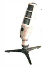
Built-in transformer gives high or low impedance: impedance is changed by altering cable connections in adapter socket plugs; high impedance sensitivity, -98 db; low impedance sensitivity, -93 db (ref. 1v/dyne/cm²); ribbon response 30-14,000 cps: British design \$66.00
