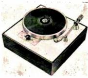
2-speed: 331/3 and 45 rpm; 4-pole induction motor; 12" aluminum turntable; rubber mat; rim-driven by idler wheel; noise level: 40 db below average recording level; built-in for 45 rpm records; stroboscopic disc; dimensions for cabinet installation: left to right 16/2", front to back 16/4", height above deck 3", height below deck 5/4"; finish: silvertone aluminum; also available Model L-37 (331/3 and 78 rpm)......\$59.95 Net L34H (with hysteresis synchronous motor)
