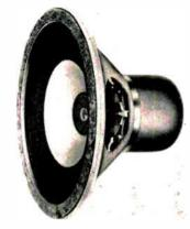
12" woofer: cone resonance 30-35 cps; total flux 240,000 maxwells; 3" voice coil diameter; power rating 35 wats
