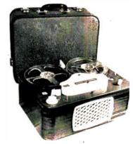
Two speed (11% ips and 33/4 ips) dual track; wow and flutter below .2% at 33/4 ips and below .25% at 11% ips; frequency response 50 to 8,000 cps ±2 db at 33/4 ips and 50 to 4,000 cps ±2 db at 11/8 ips; signal-to-noise -57 db at 33/4 ips and -54 db at 11/8 ips; hum level -52 db at both speeds; record-playback head has .00025" gap; erase and bias frequency 331/3 kc; record amplifier distortion below 1%; playback amplifier distortion below 5% at full output of 3.3 watts; included is
