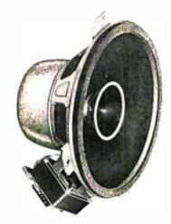
12" coaxial speaker; frequency response 30-18.000 cps; peak power rating 20 watts; built-in crossover network; crossover point 1,000 cps; impedance 4 ohms; 11.2 lbs. \$69.75
