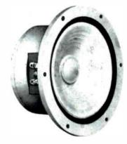
Frequency range 300-6000 cps; uses plastic diaphragm and foam suspension; power 25 watts; impedance 8 ohms.
