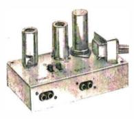
Stereo preamplifier; designed primarily for conversion from ceramic to magnetic cartridges where preamplification is not available; channel separation better than 40 db; 47,000 ohms input impedance; low impedance output; sensitivity 4 mv for 0.4 volts output; self-powered \$24.95
