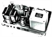
Ultra-linear power amplifier output 60 watts (130 watts peak); Acro TO-330 output transformer; 5 to 100,000 cps ± 0.5 db at 1 watt, 15 to 35,000 cps, ± 0.1 db at 60 watts; harmonic dis-tortion 0.5% (20 to 20,000 cps at 60 watts ± 1 db); intermodulation dis-tortion 1% at 60 watts (60 and 6,000 cps at 4:1). 0.5% at 50 watts; noise level -90 db; sensitivity 0.55 volt input for 60 watts output; 4, 8 and 16 HF-60 (kit).....HF-60 (factory wired)... \$99.95
