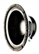
12" speaker: ceramic magnet structure produces over 1,000,000 maxwells; frequency response 16-4000 cps; 2-piece cone construction; capacity 35 watts; \$59.00 16 ohms impedance.....
