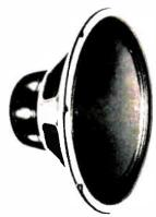
15" woofer; 83'8" deep, 131'4" diameter 2,000 cps in "Imperial" horn, 30 to 2,000 cps in Bass Ultraflex, bass reflex, and others; 16-ohms impedance; 3½ lb DP-Alnico-V magnet; resonance 35 cps; viscous edge damped diaphragm. ....\$56.80 Net
