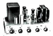
Power output 50 watts (100 watts peak); 20 to 30,000 cps ± 0.1 db at 50 watts; harmonic distortion 1% 20 to 20.000 cps within 1 db of 50 watts; intermodulation distortion 1% at 50 watts, 1/2% at 20 watts (60 and 6,000 cps at 4:1); hum and noise on magnetic phono -60 db, tuner -75 db; sensitivity; magnetic phono, 8 milli volts for 50 watts output, tuner, TV, tape, auxiliary 0.6 volts for rated output; 4, 8 and 16 ohms output impedance; 2- EL34/6CA7, 2- ECC83/12AX7, ECC90/6C4, 6CG7, GZ34;
