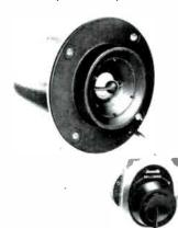
Domed phenolic diaphragm and spherical diffractor; high compliance; frequency response 3-44kc; 120° dispersion; 45%" diameter; built-in crossover network; 3 lbs......\$24.95
