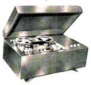
Monaural and stereo playback unit with provision for adding single or dual recording preamplifiers, 7½ ips; three capacitor induction motors; 3 heads: response: 40 to 15,000 cps: flutter and wow less than 0.17%, push-button and level controls; cabinet finished in blonde or mahogany with removable lid; 251/2"w x153/4"d x12"h. .......\$395.00 .....\$395.00
