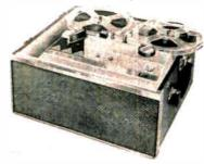
4-track, 2-track stereo play: mono record/play; 2 speeds (3¾, 7½ ips) frequency response 100-10,000 cps at 7½ ips; wow and flutter less than 0.3% volume and tone controls; 1 high impedance input; 2 outputs: 4 ohms speaker output and preamplifier output: 3-position function control: record, idle, play; wind rewind; speed selector pushbutton; self-contained 5" woofer, 4" tweeter; needs Model SP601 amp/ speaker for 2nd channel playback; crystal microphone; 14" x 81/4" x 127/8: 17
