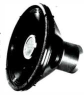
quency response: 30 to 15,000 cps; resonance: 40.45 cps; impedance: 15 ohms; crossover frequency: 2,000 cps; woofer magnet weight: 3½ pounds Ticonal G: tweeter magnet weight: 2½ ozs. Ticonal G: flux density of woofer: 16,000 gauss: flux density of tweeter: 15,000 gauss; recommended enclosure: 6 cubic feet; weight: 14½ pounds.
