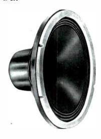
Wide range single cone 8" speaker; power rating: 15 watts average, 25 watts peak; frequency response in suitable enclosure: 35 to 14,000 cps; impedance 8 ohms; 28.5 oz. ALNI magnet; serves as single full range speaker or as woofer in conjunction with LP-65 tweeter and HP-1 high pass filter: baffle opening required 71/4"; depth 4"
