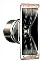
Compression type driver with horn; frequency response to 19 kc; 16 ohms impedance; sensitivity 57 db; 8 oz magnet; crossover 3500 cps; size 2"h x51/4" w x 31/4"d; driver diameter 21/4"; shipping weight 3 lbs \$35.00 Model T35B frequency response to 18 kc; 4 oz magnet; for lower efficiency systems ....
