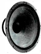
12" woofer: power rating 50 watts: frequency response 15 to 5.500 cps for 10:1 average loudness range; impedance 8 ohms: free air resonance 30 cps ±5 cps; total air gap flux 110,000 maxwells; diameter 121/4"; depth 5%2".
