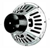
12" full range speaker; power rating 15 watts: frequency response 50 to 12,000 cps; resonance 75 cps; 1" voice coil; 6.8 oz. magnet....
