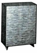
Ducted port design enclosure; 23" w. x 30" h. x 13" d.; 4.3 cubic feet; 1/2" 5-ply pyroxylin covered plywood; fiberglass acoustic padding: Acoustone plastic grille cloth; 15" or 12" woofer and separate tweeter or coax speaker; 15"-12" reducing ring, tweeter port cover.
