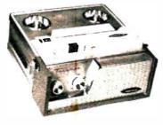
Push-button operation; plays/records 4 or 2-track tape; electronic record level indicator; wind or rewind 7" reel in 80 sec; speakers: 4"x6" oval with built-in cone, 4" round PM; frequency response 40-15,000 cps. at 71/2 ips, 40-12,000 cps. at 3¾ ips.; monitor switch and speed change while playing; tubes are 6-7025, 12AT7, EM840, 2-6AQ5, 6x4; 61/2"x121/4"x121/6"; 18 lbs.
