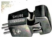
Designed for record changers; frequency response 30–15,000 cps; channel separation more than 20 db at 1,000 cps; output 5 mv per channel at 1,000 cps; recommended load 47,000 ohms; 4 terminals: tracking force 5-8 grams; standard mounting; 0.7 mil diamond ... \$16.50 Model N8D diamond stylus.....\$8.25
