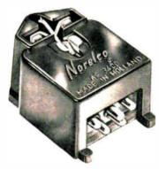
"Magneto-Dynamic" design; frequency response, frequency response flat from 50 cps to 18 kc; output, 30mv per channel at 10 cm/sec; vertical compliance, better than  $3.5 \times 10^{-6}$  cm/dyne; lateral compliance,  $4.5 \times 10^{-6}$  cm/dyne; channel separation, better than 22 db at 1.000 cps; moving mass, 2 mg; stylus pressure, 3-5 grams; complete with 0.7 mil diamond stylus, mounting plate and hardware
