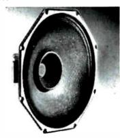
8". twin cone: capacity 6 watts: frequency response: 75 to 19.000 cps; impedance 4-6 ohms: total magnetic flux 26.000 Maxwell: flux density 11.000 gauss; efficiency 6% at 400 cps. \$9.90 Net
