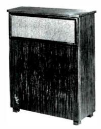
Enclosure uses resistance damped Helmholtz resonator; frequency response 50 to 15,000 cps; 2-way, 3-speaker system; built-in electrical crossover at 6,500 cps; 8" bass and midrange speaker; 2 cone-type tweeters; uses system of distributed slots to increase resistance damping: impedance: 8 ohms; power rating: 20 watts: size: 33¾"h x25¼"w x11"¾d; mahogany, blonde, or walnut laminate finishes
