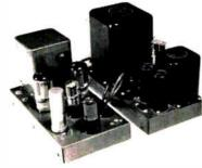
Rated output: 20 watts, 36 watts peak; dual chassis Williamson type circuit; frequency response: 6 to 150,000 cps ±1 db at 1 watt; harmonic distortion: less than 1% at 20 watts: IM distortion: less than 1.3% at 20 watts; sensitivity: 1 volt for 22 watt output; hum and noise 88 db below rated output; output impedances: 4, 8, 16 ohms; damping factor: 14; tubes: 2-6SN7GT, 2-5881, 5V4G; Acrosound TO-300 output transformer; each chassis 7"h x 5½"w x11"l. .....\$49.75
