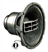
Coaxial two-way systems; Model H-222 is 12"; response 30 to 15,000 cps; 16ohms impedance; 134 lb DP Alnico-V magnet; compression driver horn-loaded tweeter with crossover at 2,000 cps; high-frequency balance control; requires baffle opening 10½"; has 8¼" depth. H-222......\$62.50 Net
