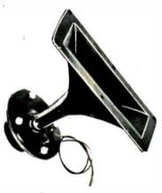
Compression type tweeter; cloth base plastic diaphragm; 20 watts; 2.000 to 15.000 cps; 16.0hms impedance; shipping weight 2½ lbs; 3"x7½"x6½"; baffle cutout 6"x2" ......\$16.50 Net
