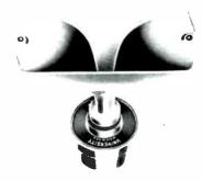
One-piece die-cast horn with 120° horizontal and 50° vertical dispersion: hermetically sealed construction; response from 2000 to 15,000 cps; 8 ohms; power rating 25 watts; 6"x23/4"x65/16". \$18.00 Net
