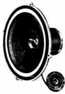
Main cone is foam suspended producing response below 30 cps.; Tweeter assembly is paper core suspended in foam, aluminum center dome, aluminum voice coil: capacitor protects tweeter from low frequency input below 4 kc.; volume control attached to tweeter; 2 magnet gaps of 134" and 1": 12 watts input; impedance 12–15 ohms; baffle opening 1078": depth 7"; weight 26 lbs...\$139.50
