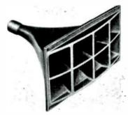
Supplied without driver: cut-off 600 cycles; disperson angle 120°; requires panel opening 5" x 103/8"; dimension 11" x 6" x 11" deep.....\$17.00
