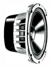
8" high compliance dual voice coil woofer; frequency response 38-2,200 cps; power rating 30 watts: impedance 8 ohms; 41/4" depth.....
