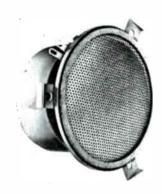
Armored horn type tweeter with plastic cone; overall diameter  $2\frac{1}{2}$ "; frequency response 2,000-18.000 cps.; 2 watts peak power; 5.5 ohms impedance \$8.50
