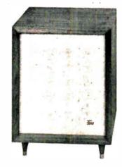
Folded horn enclosure; frequency response: 40 to 15,000 cps; two-way system with horn-loaded tweeter; 800 cps constant resistance crossover network with 12 db/octave attenuation; 241/4"w x30"h x161/2"d ......\$290.00
