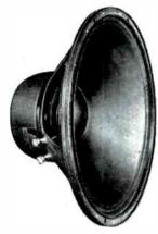
15-inch woofer: power rating 30 watts; 16-ohms impedance; 2.7 pound Alnico V ring magnet; special rim compliance prevents cone breakup; 3-inch diameter copper ribbon voice coil is wound; cast aluminum edge-wise frame.
