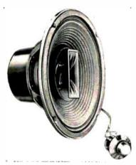
12" three way; capacity 20 watts; frequency response 35 to 15,000 cps (in E-V Aristocrat enclosure); resonance 45 cps; 16 ohms impedance; sensitivity 46 db; magnet 18 oz.; built-in crossovers; mechanical 2000 cps; electrical 3500 cps; depth 61/16"; shipping weight 14 lbs.
