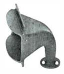
Cast aluminum exponential horn used with JBL 175 and 275 drivers in systems crossing over 600 cps and above: geometry of throat area gives smooth distribution of high frequencies.......\$37.50
