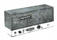
40 watts power, up to 80 watts peak; less than 1% IM distortion at 40 watts; frequency response ±0.5 db. from 10 cps to 40 kc.; sensitivity 1.3 volts rms. input for 40 watts output; output impedances are 4, 8, and 16 ohms; tubes, 2—EL34, 7199 GZ34 selenium rectifier; 5" x 14" x 61/2" .....
