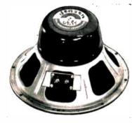
12" woofer; 7" deep, 101/2" diameter baffle cutout required; single cone; 25 watts; 30 to 2,000 cps, resonance 55 cps: 16-ohms impedance; 134 lb DP Alnico-V magnet: viscous edge damped diaphragm; shipping weight 10 lbs. .\$36.50 Net
