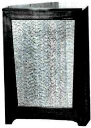
Folded corner horn design; frequency response: 40 to 22,000 cps. with substantial efficiency from 60 to 16.000 cps, down 10 db at 49 cps; three-way, three-speaker system; built-in electrical crossovers at 1.000 and 5,000 cps; uses Stephens or Electro-Voice 15" or 12" bass
