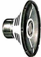
Coaxial units; K-80 is 10", 12 watts, Coaxial units; K-30 is 10, 12 wats, 16 ohms, response 50 to 14,000 cps; K-210 is 12", 14 watts, 8 ohms, response 45 to 14,000 cps; K-310A is 16 watts, 16 ohms, response 40 to 14,000 cps; Models K-80 and K-210 use ½ lb DP Alnico-V magnet; K-310A uses 3/4 lb DP Alnico-V magnet; coaxially mounted direct radiation cone-type tweeters; K-310A has high frequency balance control as standard equipment. .....\$17.75 Net .....\$27.50 Net K-80A. K-210 \$39.75 Net K-310A
