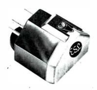
Two d'Arsonval moving elements; vertical and lateral compliance  $5x10^{-6}$  cm/dyne; output per channel 6 mv at cm/sec: frequency response 18-20,000 cps; fits any standard arm; Model P99 designed for use with Model ESL—S310 arm.
