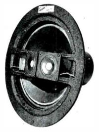
Coaxial speaker; 15" mounting frame; depth 7": 15 watts continuous, peaks to 30 watts; 40 to 16,000 cps; 8-ohms impedance: composed of B-199A woofer and B-200X twin-tweeter: crossover at 2,500 cps; fits standard cutouts for 12" and 15" speakers; infinite baffle enclosure recommended, minimum 5 cubic feet, optimum 9 cubic feet.
