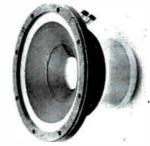
8" single-cone wide range speaker; power rating: 25 watts continuous, 50 watts peak; frequency response: 40 to 15,000 cps; impedance: 16 ohms; magnet weight: 1 lb: free air cone resonance: 50 cps: 2" aluminum voice coil; plastic impregnated cone suspension; curvilinear cone; diameter: 81/4"; depth: 41/4" \$33.50
