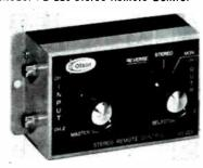
Provides master control of both channels from single knob and selects stereo stereo reverse, or monaural; connects between program source and amplifiers; input and output connections terminate in RCA type phono jacks. .....\$3.00
