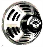
12" wooser; 61/16" deep, 101/2" diameter baffle cutout required; 20 watts; 40 to 2.500 cps; 16 ohms impedance; resonance 60 cps, viscous edge damped diaphragm. ..\$12.90 Net
