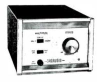
For use with Crosby Multiplex System; controls for level, split-circuit, stereo balance: detector bandwidth ±30 kc; subcarrier sensitivity 2 mv: output 1 volt: frequency response ±1 db 20-20,000 cps; tubes are 12AU7. 12AX7, 7199. 6BF6. selenium rectifier: 53/4" x 101/2" x 4" \$60.50 Model AMX (plug-in no power supply) \$49.50
