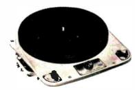
Three speed transcription turntable; 4-pole shaded motor; dynamically balanced armature; rotor set into phosphor bronze bushings; 12", 61/2 lb. cast aluminum turntable; rubber mat; wow less than 0.2%; flutter less than 0.5%;
