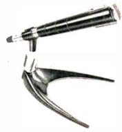
Dynamic type; frequency response 60-12,000 cps.; high and low impedance models; output -57 db. at 1 volt/dyne/ cm.2; complete with lavalier and stand adaptor; 8' extra shielded, single conductor cable.
