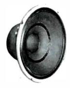
8-inch Biflex cone-type speaker with second compliance ring in the center of the cone to give mechanical cross-over at 1.000 cycles and permit 2-way performance with a single voice coil; 15 watts: 60 to 16,000 cycles; 8-ohms impedance: Alnico V ring magnets: mechanical crossover at 1,000 cycles.
