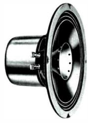
8" wide range Diffaxial speaker: frequency response 45-14,000 cps; power rating 25 watts; mechanical crossover at 5,000 cps: impedance 8-16 ohms; 41/4" depth .\$16.95
