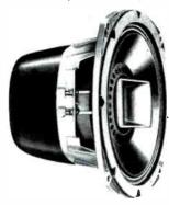
Employs compression tweeter and 8" woofer: mechanical crossover at 1000 cps and electrical at 5000 cps; response to 15,000 cps; power rating 35 watts; 8-16 ohms; 5½" deep.......\$42.00 Net
