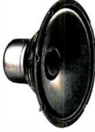
Model UX-80 is 8", 614" depth; Model UX-120 is 12", 8½" depth; UX-80 is 12 watts, UX-120 is 14 watts; frequency response 40 to 12.000 cps, resonance 55-60 cycles; 8-ohms impedance. ½ 1b DP-Alnico-V magnet; single cone wide range. single cone wide range. UX-120 .... .....\$17.95 Net
