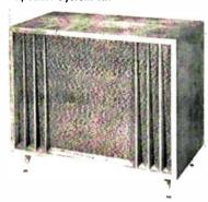
Modified infinite baffle enclosure: frequency response; 25 to 20,000 cps; power rating: 50 watts of program material; impedance: 16 ohms: 3-way, 3-speaker system: two Altec 15" low frequency drivers, one Altec high frequency driver with special horn: speaker magnet weights: low frequency drivers, 2.4 lbs each: high frequency driver. 1.2 lbs.; "M" derived parallel filter type dividing network with 500 cps crossover: 34" plywood; 41"w x2234"d x 34"h \$\frac{34"}{299.95}\$
