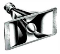
Mid-range and high frequency horn with 600 cps cutoff; die-cast design with reciprocating flare design for uniform dispersion; fits any driver with standard 13/8"-18 throat... .....\$19.00 Net
