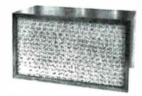
Acoustic suspension two-way system; 42-14,000 cps ± 5 db; down 10 db at 30 and 16,000 cps; 10-inch woofer and special tweeter; built-in crossover; 8 ohms impedance; harmonic distortion at 10 watts under 2% to 60 cps, under 3% to 50 cps; recommended amplifier power; 20 to 40 watts; bookshelf type: 13½"x24"x11¾"; 33 lbs.; hardwood veneer.
