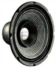
Model DX-120 is 12", Model DX-150 is 15": DX-120 is 20 watts. DX-150 is 22 watts: response 40 to 13,000 cps, resonance 48-50 cps; 16-ohins impedance: 1 lb DP-Alnico-V magnet: dual cones; mechanical crossover at approximately 4,000 cps; single voice coil. .\$27.50 Net DX-120 .
