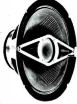
coaxial speaker: power rating: woofer, 50 watts: tweeter, 32 watts: frequency response 30 to 17,000 cps for 10:1 average loudness range: impedance 8 ohms: free air resonance 50 cps ± 5 cps; total air gap flux; woofer, 110.000 maxwells: tweeter, 18,000 maxwells: dispersion 115 degrees; diameter 12½": depth 5½2"......\$59.95
