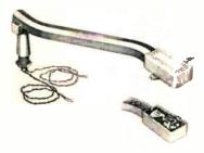
Economy unit; all plastic manual tone arm; available with compression rear mount or solid rear mounting post; tracking force 9-11 gm; includes new Model 12 crystal cartridge.......\$7.45
