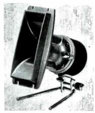
Die cast horn tweeter using "recipro-cating flare" principal for wide angle dispersion; 20 watt driver unit coupled to horn provides uniform response from 2,000 to above audibility: 8 ohms:  $2'' \times 4\frac{3}{4}'' \times 5\frac{1}{2}''$  \$8.95
