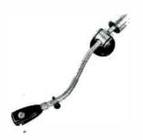
For use with stereo and monaural cartridges; ball bearings used throughout for all vertical and lateral movements; rotationally balanced, tracks at up to 90 degree angle: tracks at 2 grams when used with ESL C-100 cartridge.....\$34.95
