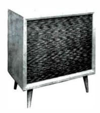
Bass reflex design; accommodates 2- and 3-way speaker systems; cut outs for 15" and 8" speakers with daptor boards for 12" and 5" speakers: size: (less 7" legs) 287/8"w x231/2"h x163/4"d; 3/4" birch; finishes: mahogany, blonde.
