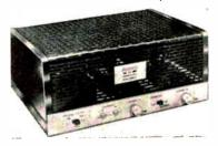
Dual 18-watt amplifiers on one chassis; may be used for stereo or monaurally (36 watts output); frequency response 35 to 30.000 cps ±0.5 db; harmonic and IM distortion less than 1%; input sensitivity per channel: 0.45 volts for full output; tubes are 2—6AN8, 4—7189, GZ34; 9½6"x5½"x13½"...\$44.50
