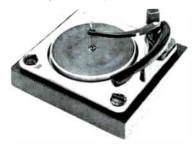
4-speed intermix record changer; 4-pole induction motor; rim-driven turntable with automatic idler disengagement and rubber mat; wow and flutter less than 0.25% rms at 33½ rpm; transcription-type tone arm maintains equal stylus pressure from bottom to top of record stack; manual operation switch; automatic shut-off after last record; muting switch and condenser......\$49.50
