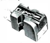
Ceramic-type cartridge for stereo or monaural records; frequency response 30 to 20,000 cps, within 1.5 db from 30 to 7.000 cps; compliance (vertical and lateral) 2 x 10<sup>-6</sup> cm/dyne; output voltage 0.4 volts; conforms to RIAA curve; recommended stylus force 5-7
