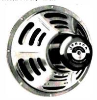
Extended range speakers: P10-SX is 10", 51.4" deep, 83.4" baffle opening required; Model P12-SX is 12", 61/16" deep, 101/2" baffle opening required; P10-SX is 12 watts, P12-SX is 13 watts; 8-ohms impedance; 4.64 oz Alnico-V magnets in both models; 1" diameter voice coils. P10-SX \$9.58 Net
