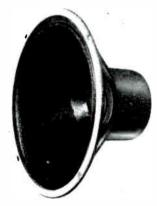
12" woofer; 51/8" deep; variable density cone; 15 watts, 30 watt peaks; 40 to 4,500 cps: 8-ohms impedance, 16 ohms on special order: 11/2-lb. Alnico V magnet: unique voice coil construction; cast aluminum frame.
