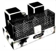
Seventy-watt power amplifier: frequency response at 1 watt 10 to 100,000 cps ±1 db; harmonic distortion less than 2% 20 to 20,000 cps within 1 db at 70 watts, less than 1% at 60 watts; IM distortion below 1½% at 70 watts, below 1% at 60 watts; damping factor
