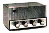
Power output 12 watts, 20 watt peaks; sensitivities: tuner—.75 volts, mag. phono—4.5 mv., microphone—5.5 mv.; IM distortion 3% at 12 watts; frequency response 40-30,000 cps.; tubes are 2-12AX7, 2-6V6GT, 5Y3GT; 91/2"x61/4"x61/4"; 12 lbs.....\$29.95
