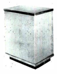
E-300 infinite baffle enclosure: 3/4" plywood with mahogany, walnut or birch veneer; speaker is the B-207A coaxial; 40-16,000 cps; 2,500 cps crossover; handles 15-watts continuous, peaks to 30 watts; 8-ohms impedance; has provisions for adding B-209 mid-range speaker; 24"w x17"d x301/2"h; 60 lbs. B300 Contemporary (Enclosure
