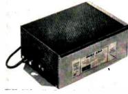
Consists of two two-stage neutralized amplifiers; one for FM plus low band; the other for high band VHF. Input and output impedance is 300 ohms; bandwidth—54-108 mc; 174-216 mc;
