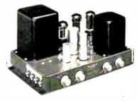
Rated output: 20 watts; built-in preamp: two-position record equalization; bass control: 15 db boost or cut at 30 cps; treble control: 15 db boost and 20 db cut at 15,000 cps: frequency response: 20 to 20,000 cps ±1 db; harmonic distortion: 1% at 20 watts; inputs: magnetic (7 millivolt sensitivity), mike, crystal phono, tuner: output impedances: 4, 8, 16, 500 ohms; tubes: 12AX7, 2-12AU7, 2-6L6G, 5V4G; 14"x8%"x73%" high .......\$35.50
