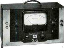
Tape recorders produce flutter and consequent frequency modulation noise for many reasons and it is impossible to perform the adjustments necessary to maintain high quality reproduction without a flutter meter.
