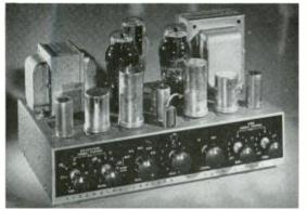
The AR-420 has a complete but simple preamp-control section.
