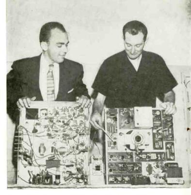
No more "jungle" of wires. Chief Engineer Fred Miller (right) makes a side-by-side comparison of a Walsco PC-9 (right) with a conventional, complicated chassis. Bob Mueller, Walsco Sales Manager, observes simplicity of vertically mounted, printed circuit design.
