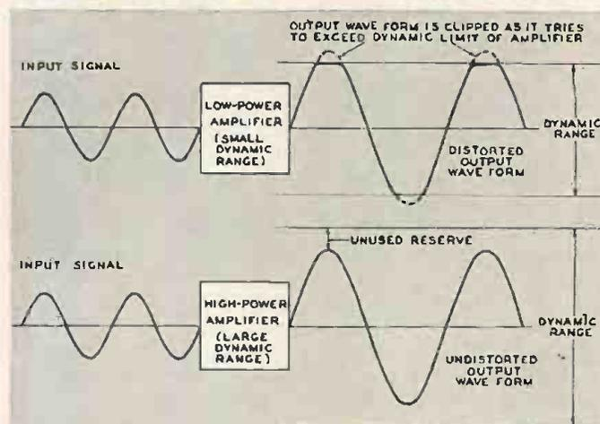
Fig. 2-4. Two identical signals applied to low-power and high-power amplifiers. The signal is too large for the low-power unit, causing it to overload and distort. The high-power amplifier handles its signal easily, with a safety margin; output signal is undistorted.
