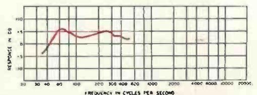
This is E-V phase loading. As you can see, performance in an along-the-wall position closely approaches that of the corner horn.
