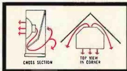
The folded corner horn drawings here show sound path from direct radiators.
