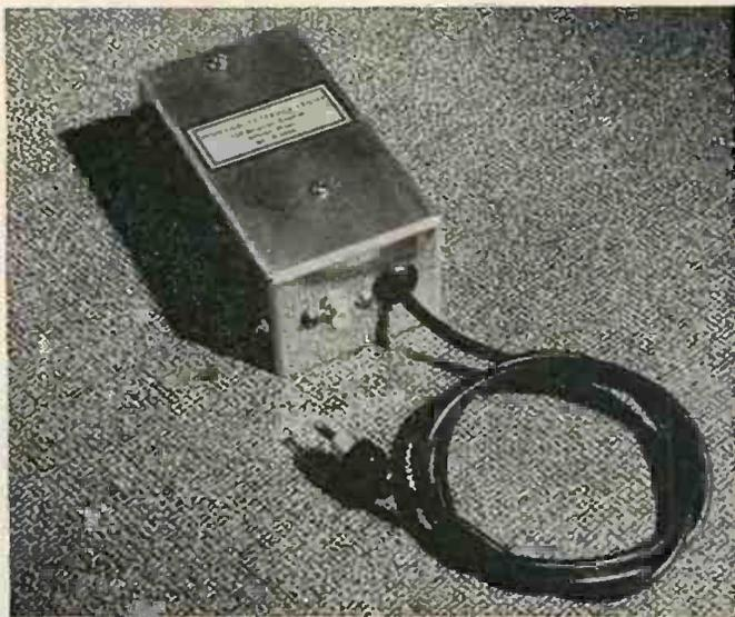
*The booster connects between pickup and preamp.*
