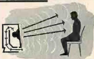
KwiKit acoustic design and tilted baffle combine direct speaker radiation and compensated rear horn loading in a way that blends bass, middle and treble ranges perfectly... for uniform response throughout the listening areas of a room.
