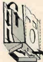
Underside view shows how advanced design, self-contained folded horn extends to the front of the cabinet, projecting low frequencies out into the room... not back into a corner, splashed against the walls. Small slot in base is resistively controlled vent which equalizes woofer diaphragm excursions in compression chamber. KwiKits are therefore independent of room furnishings, shape or placement and can be used against a flat wall, in a corner... even up in the air!
