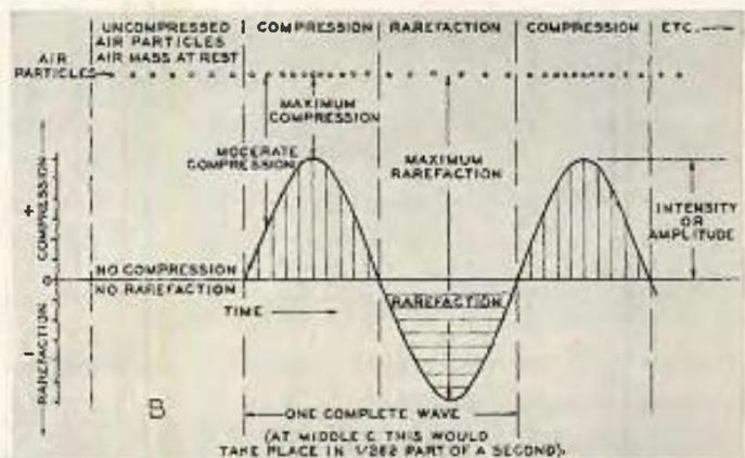
Fig. 2-1A, above: how a sound wave is produced. A vibrating string or diaphragm compresses the air particles in its path, and rarefies them in back. Fig. 2-1B, right: graphic picture of a sound wave.
