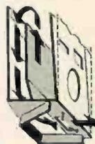
Underside view shows how advanced design, self-contained folded horn extends to the front of the cabinet, projecting low frequencies out into the room... not back into a corner, splashed against the walls. Small slot in base is resistively controlled vent which equalizes woofer diaphragm excursions in compression chamber. KwiKits are therefore independent of room furnishings, shape or placement and can be used against a flat wall, in a corner... even up in the air!
