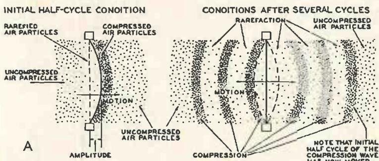
Fig. 2-1A, above: how a sound wave is produced. A vibrating string or diaphragm compresses the air particles in its path, and rarefies them in back. Fig. 2-1B, right: graphic picture of a sound wave.
