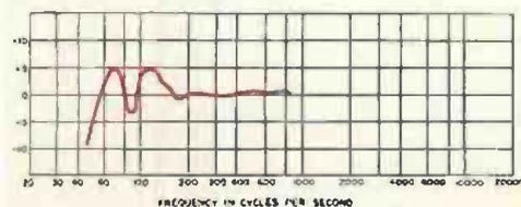
This curve shows performance of the usual 4-way systems in a bass reflex cabinet. Note the dip at 85 cps, which shows the destructive cancellation and the reinforcement (peak) at 120 cps which causes "boom."
