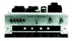
**THE EQUIPMENT:** Fisher X-101-C. a combination stereo preamp/power amp. Chassis dimensions: 15 1/8 inches wide, 12 1/2 inches deep, and 4 13/16 inches high. Price: \$199.50. Optional metal case, finished in simulated leather: \$15.95; wood (mahogany or walnut) case: \$24.95. Manufacturer: Fisher Radio Corp., 21-21 44th Drive. Long Island City 1, N.Y.
