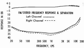
show some increase, but in the Model 18 this increase was virtually nil, Channel separation on stereo was excellent, and stereo response was virtually perfectly flat across the FM audio band, showing no appreciable difference from the set's mono response. Both channels, too, were very closely balanced, Calibration of the tuning dial was highly accurate. Other measured characteristics, shown on the accompanying chart, simply add up to a really first-rate tuner.
