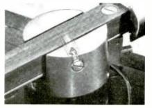
...to the correct fraction of a gram. Because of today's featherweight tracking, the slightest interference with free arm movement may affect the cartridge's performance. To avoid this, the Lab 80 arm moves on needle pivots, set into tiny ballbearings. Flat arm geometry cancels warp www: low center of gravity eliminates sensitivity to external jarring.
