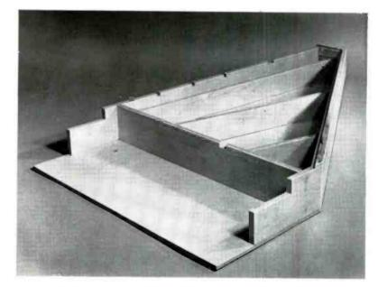
The inner case, made from 3/4-inch plywood, is the first stage of construction. It's a good idea to place all side pieces and three braces loosely on top of the plywood bottom in position they are to occupy. This gives one a chance to check for errors in measurements. Be sure the two mitered corners fit accurately. Next step is to glue and screw boards in place. For all gluing operations a white glue is used. Allow half an hour for drying.
