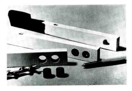
Keys need lead weights inserted to fall back after having been depressed. Holes are drilled from side to side, and then plugged with lead weights. All the white keys require two pellets, while black keys need only one slug. A prick punch was used to tamp leads enough to gain a sufficient spread to hold lead in keys.
