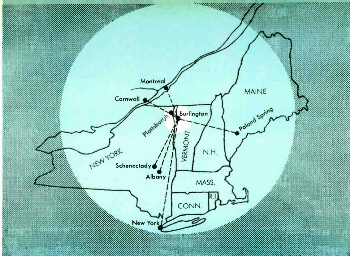
In the Burlington, Vermont area only two TV channels could be received prior to the cable, as shown in the small center area which represents a 30-mile radius. The Green Mountain cable system has expanded TV coverage by ten times that distance. A channel now is received from each city shown, with Montreal supplying three TV plus three FM channels. Response to the system has been so encouraging that Burlington CATV operators are launching their own local educational channel too.
