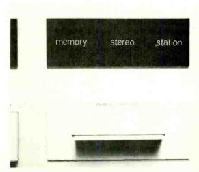
When punched card is inserted in Scott's "memory" slot, it overrides scanning control and lights "memory" indicator on the enunciator panel above the card slot.
