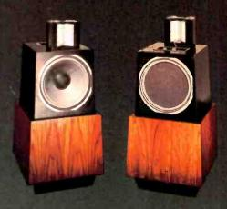
Beneath its grille cover the ESS amt 1a features all new components. On its front panel is the powerful new 12 inch woofer and above it the latest configuration of the revolutionary Heil air-motion transformer. The rear panel mounts the flat surfaced neoprene and styrofoam passive radiator. On the top surface, behind the Heil airmotion transformer, is the recessed panel with controls for midrange and treble response that adjust for differing room characteristics.
