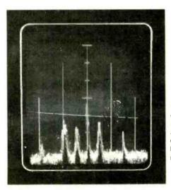
"Panoramic display" here shows four weak stations on adjacent channels (200 kHz apart), alternatechannel spacing between two at right.
