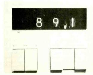
Scott's scan modes are controlled by these pushbuttons. Bidirectional scan is an important feature for easy use; channel mode stops at both odd and even decimals.
