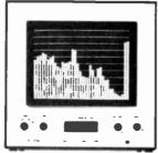
The B&K real-time analyzer: controls (at left) and readout.
