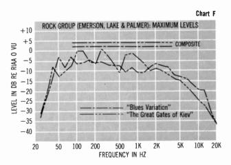
Composite musical curves prepared with the B&K analyzer. A, B, and C represent three movements of *The Planets* by Holst. Two movements of the Dvořák *American* Quartet, Op. 96, are shown in D. E and F show sections from *Pictures at an Exhibition*, rendered by Emerson, Lake, & Palmer.
