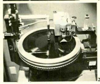
used for 12-inch LPs are 14 inches in diameter while 45s are cut on 10- to 12-inch discs; the extra size not only provides a banding sample to check signal-to-noise and groove geometry, but also facilitates easier handling in plating (the next step).
