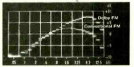
Real-time analysis of Dolby FM receiver output when tuned to interstation noise, using Alfec Hewlett-Packard 8050A analyzer. In a "perfect" FM system the trace would be a continuously rising straight line. Thus the results show that highly modulated high-frequencies can be reproduced with significantly improved accuracy using Dolby FM.
