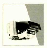
M24H . . . the carridge that does not compromise stereo reproduction to add four-channel capability. Superb stereo trackability and quadriphonic carrier signal retrieval. New hyperbolic stylus tip, high energy magnet, and low-loss laminated electromagnetic structure. 1 to 1-1/2 gram tracking force.
