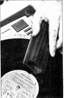
Setting up a turntable so that the pickup/tonearm combination will track the record with the lowest possible distortion is critical. In terms of getting the geometry correct, I've been pleased with the ADC Pro/Trac, which checks the lateral tracking angle at two places on the disc rather than just one. Vertical tracking force settings on many tonearms are inaccurate, so we always double-check VTF with the Shure SFG-2 gauge.
