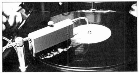
Heavy-duty record cleaning at WFMT is handled by the Keith Monks machine (top), but for quick, on-the-spot cleaning a Discwasher brush (right) is used.
