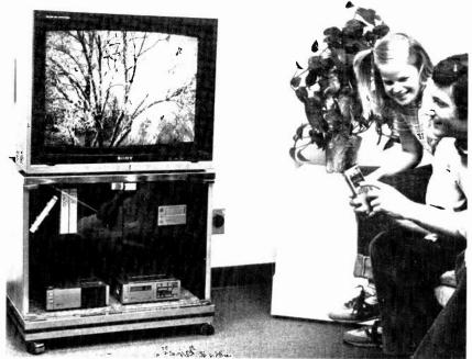
Component television systems, such as Sony's Profeel (abcve), differ from conventional sets in that they take a modular approach to maximize video and audio quality. The Profeel system consists of a video "monitor" with two built-in amplifiers, separate speakers, and a component-quality tuner.
