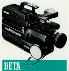
a companion tuner/timer for recording from broadcast or cable TV, camcorders include only the connections for recording from an external source. To play back tapes, most include an RF adapter (for connection to a TV set's antenna terminal) as well as direct audio-video outputs for hookup to a monitor. Some videographers may find that a camcorder's playback capabilities are sufficient to eliminate the need for a regular home VCR.
