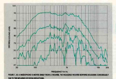
(CONTINUED FROM PAGE 55) waves and thus will not produce such jagged response curves. And narrow response peaks and dips can be inaudible, depending on their width, amplitude, frequency, and spacing across the audible spectrum. So by careful adjustment of the bandwidth of the analyzer, a rough curve can be smoothed enough to find response slopes and peaks more truly characteristic of the speaker's sound.
