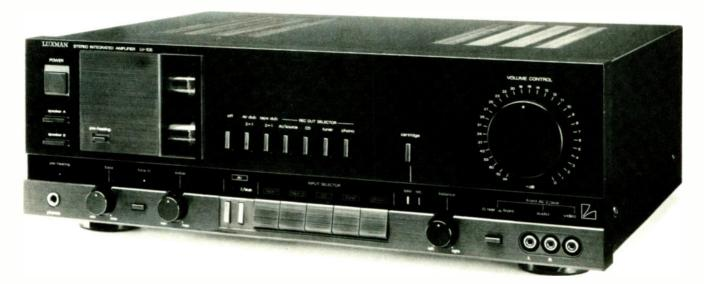
DIMENSIONS: 171/4 BY 51/3 INCHES (FRONT), 121/4 INCHES DEEP PLUS CLEARANCE FOR CONTROLS AND CONNECTIONS. AC CONVENIENCE OUTLETS: THREE SWITCHED (300 WATTS MAX. TOTAL), THREE UNSWITCHED (450 WATTS MAX. TOTAL). PRICE: \$700. WARRANTY: "LIMITED," THREE YEARS PARTS AND LABOR, 90 DAYS ON TUBES. MANUFACTURER: LUX CORP., JAPAN; U.S. DISTRIBUTOR: LUXMAN DIVISION OF ALPINE ELECTRONICS OF AMERICA, INC., 19145 GRAMERCY PLACE, TORRANCE. CALIF. 90501.
