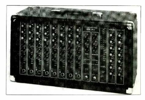
loops, two ten-LED bar graphs, two seven-band active equalizers, as well as three EQ controls for each channel. The system is also available in six and twelve channel models.
