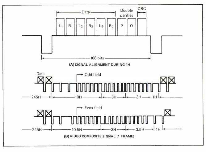
Figure 4. Retrieval of NTSC signal. A) shows the signal alignment during signal distribution on one horizontal scanning line, and B) shows one frame of composite video signal.
