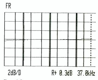
Figure 1. Frequency response of the 245F with switch set to mono. Vertical scale is 2 db/division. Sweep is from 20 Hz to 40 kHz.
