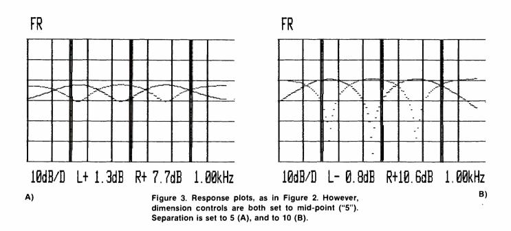
maximum setting. Note that only the amount of maximum separation has increased, while center frequencies (those frequencies at which the maximum difference in amplitude between channels occurs) remain as they were in *Figure 3A*.
