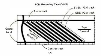
Figure 3. The NTSC TV signal is recorded on a VHS format video cassette recorder; tracks are the same as those used in video recording.
