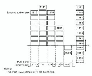
Figure 1. Sampled audio data and the resultant PCM signal.
