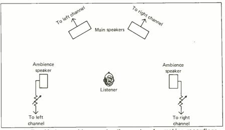
Figure 2. The Madsen ambience extraction system for making recordings sound fuller and more spacious.
