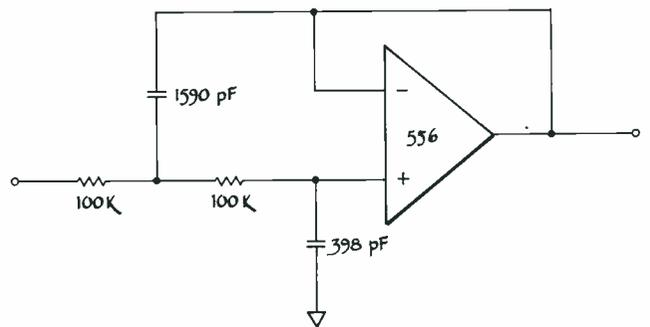
Figure 1B Butterworth Function 1KHz Low Pass Filter
