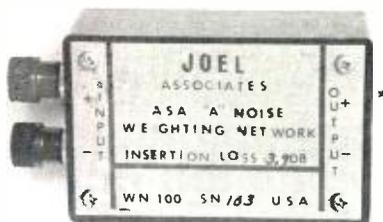
A weighted noise measurement is designed to give a response curve similar to the ear at low volume levels and is intended to give a more useful indication of the subjective signal to noise ratio than unweighted measurements.
