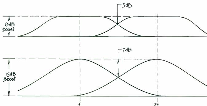
Figure 3 Bandwidth Vs. Peak-Dip Response
