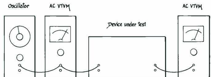
Figure 2 The usual frequency response Test Set
