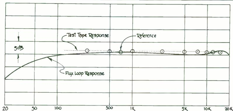
Figure 2 Comparative Response of Standard 7½ IPS Test Tape and Flux Loop
