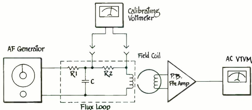
Figure 1 The Flux Loop in Calibration and Application
