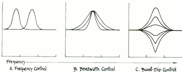
Figure 6 Parametric Equalizer Functions
