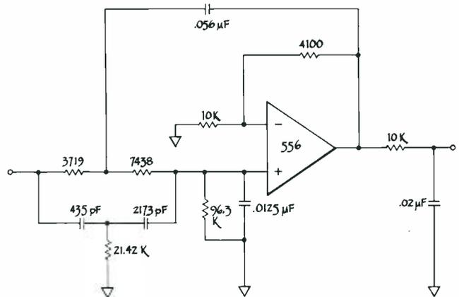
Figure 1A Elliptic Function 1KHz Low Pass Filter
