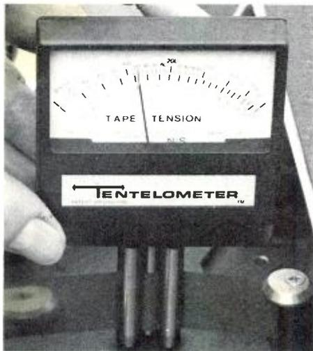
ports. TENDEL offers hand-held instruments that quickly and accurately measure dynamic or static tension on magnetic recording tape of all widths.
