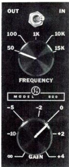
signal output from -74dBm to +4dBm. The signal generator is designed so that it may be turned on or off without introducing transients into the circuitry.
