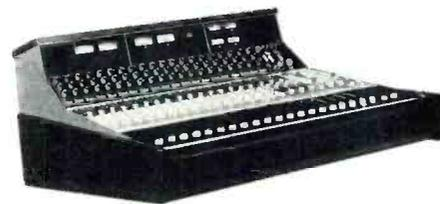
the necessary foldback, audition, intercom and program interlock features, and may be equipped with optional modules offering remote control of tape machines and turntables, or remote input pre-selection.
