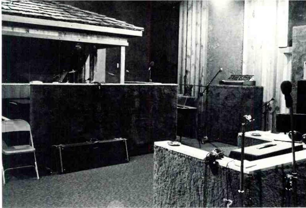
*Drum booth is placed at dead end of room as shown. Laterally dispersing sections can be seen on wall.*
