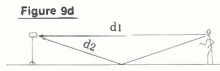
made approximately equal to  $d_2$  (Figure 9(D)) thus minimizing the comb filter effect. There are several stands and foam protectors designed to support the microphone very close to the floor surface. Another recent approach is the Pressure Zone Microphone of Ed Long and Ron Wickersham (Alembic, Inc.) enthusiastically promoted by Don Davis<sup>3</sup>.
