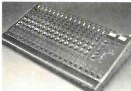
system, the Audy Series 2000 Mixing Console maintains headroom at 24 dB throughout. Other standard features include: individual channel and output patch points; transformerless balanced inputs and outputs; 3 band EQ with switchable mid-range; switchable pre- and post-monitor and effects sends; soloing for any input or output; phantom power; and work lamp socket.
