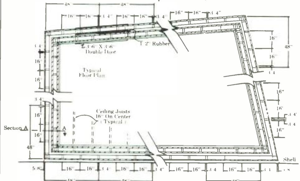
enough space, the next step is to design a floor plan (Figure 1). When laying out the sides of the room none of the walls should be parallel or even near to parallel. The ceiling should not be parallel to the floor. This is very important if the room is to have maximum random reflections and a smooth decay. It's at this stage that a bit of math should be introduced:<sup>1</sup>
