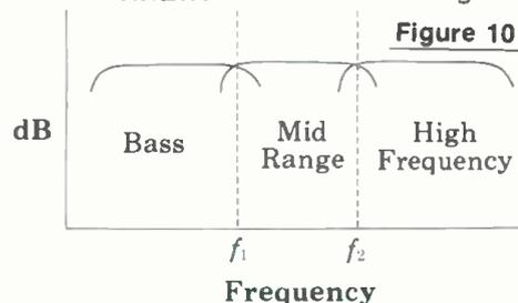
all the ingredients for generation of comb filter perturbations of response in the crossover region. The same process is active at  $f_2$  between the midrange and tweeter units. Actually a narrow band of frequencies is affected, the width limited by relative amplitudes of radiations from the two adjacent units. The steepness of the crossover curve determines the width of the frequency range affected. This is a highly
