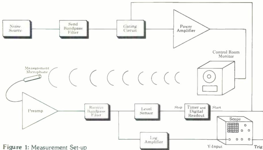
Figure 1: Measurement Set-up
