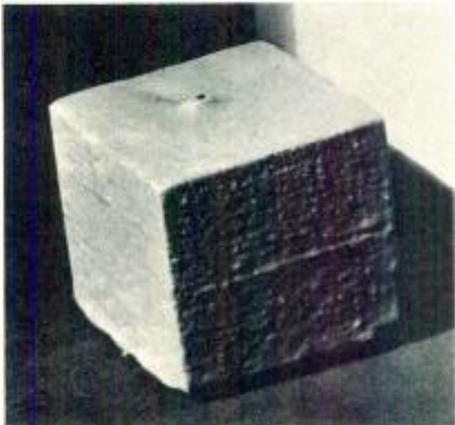
**Latex Coated Fibreglas Insulation Block**
