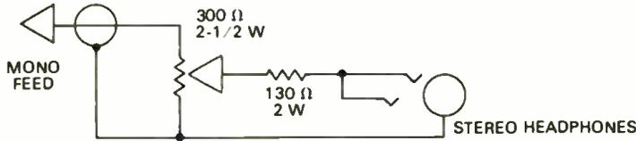
The maximum number of units is determined by the lowest impedance the amp can tolerate. With 8-ohm headphones the worst case load the box represents is 92.6 ohms. Therefore, twelve units may be used with an 8-ohm amp or twenty-four units with a 4-ohm amp.
