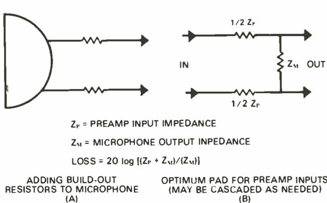
Figure 7: MICROPHONE INTERFACE NETWORKS
