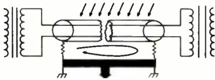
Figure 1: SHOWING GROUND LOOP INDUCTION INTO SHIELD
