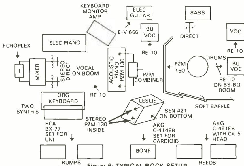
Figure 6: TYPICAL ROCK SETUP
