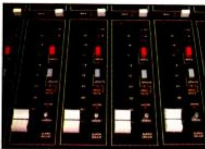
SuperGroup shows console group status at a glance, eliminating the need to scan each module.
