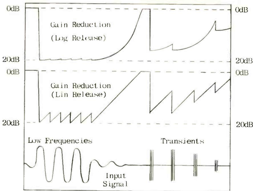
**Figure 2** — Pictographic representation of Log Response Shape vs. conventional Linear Release. Note that, although the overall release rates are similar, the Log shape produces significantly less gain modulation on low frequency material (lower distortion), and on recurring transients (less pumping and envelope distortion).
