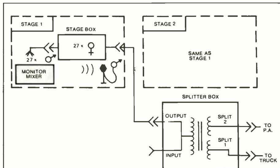
2 SETUP FOR MULTIPLE STAGES WITH INDIVIDUAL MONITOR MIXERS. NOTE "BACKWARDS" SNAKE FROM STAGE BOX TO SPLITTER BOX.
