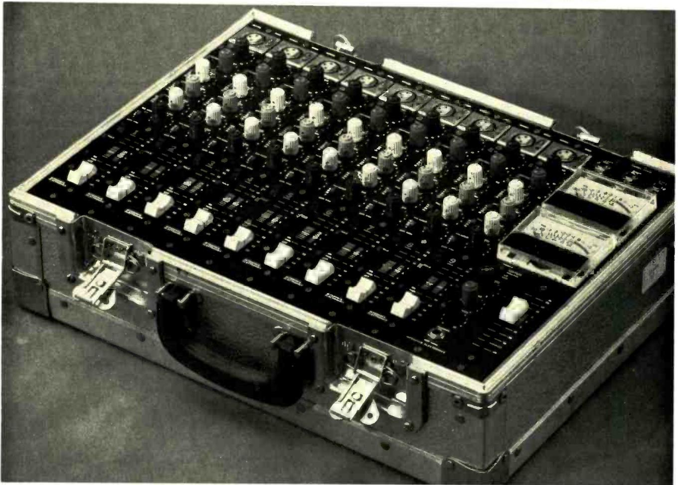
THE MODEL 200 MIXER is a special purpose compact "suitcase" portable mixer built in an ATA-style case with detachable lid and handle measuring 13 X 17.5 X 7 inches with eight or nine inputs and two stereo outputs plus echo and cue, and can be operated for 16 to 20 hours on an external rechargeable "Gel-Cel" battery (supplied, with charger). Built to the highest professional standards, it is recommended for the most exacting portable mono or stereo work.
