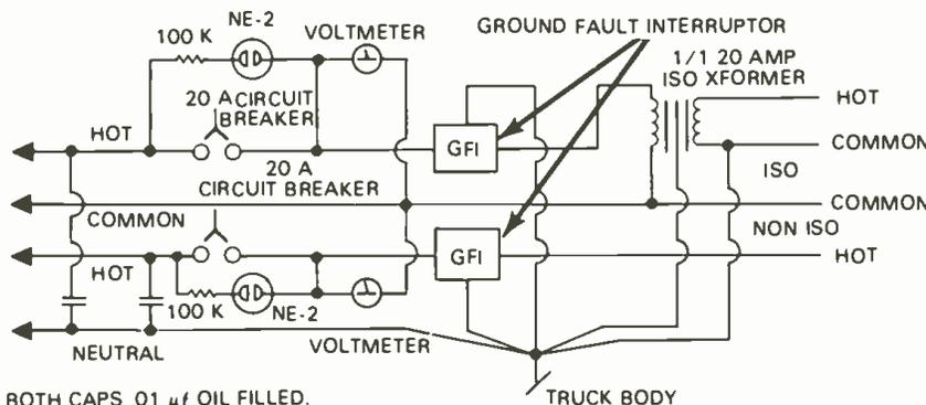
FOR SINGLE PHASE 210 VOLT POWER SEND THE COMMON AND THE NEUTRAL ARE BOTH TIED TO THE NEUTRAL BUS AT THE MAIN POWER SEND POINT.
