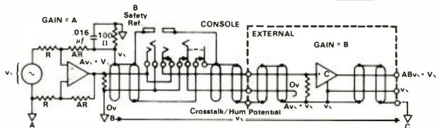
Figure 6 - Forward Referenced Amplifier
