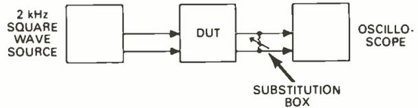
Figure 4: BASIC SQUARE WAVE TEST SETUP
