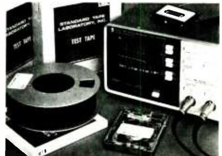
Used in conjunction with the Sound Technology system, these new tapes provide measurement of level, azimuth and frequency response of any tape or film transport. Flutter/speed test tapes also are available.
