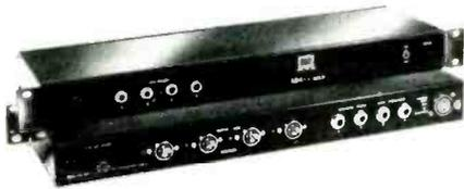
Specifications include maximum input level of +18 dBV; gain of zero to +30 dB; noise 101 dB below rated output; and distortion less than 0.2% at 20 Hz maximum rated output.
