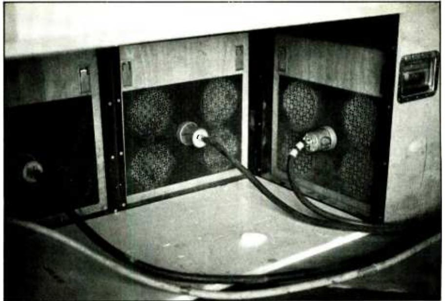
Figure 4: Clair house amp racks were positioned in tight groups of four. Intake and exhaust cooling fans were covered by a wooden enclosure, underneath which was placed a styrofoam pad that held piles of dry ice for added cooling protection.
