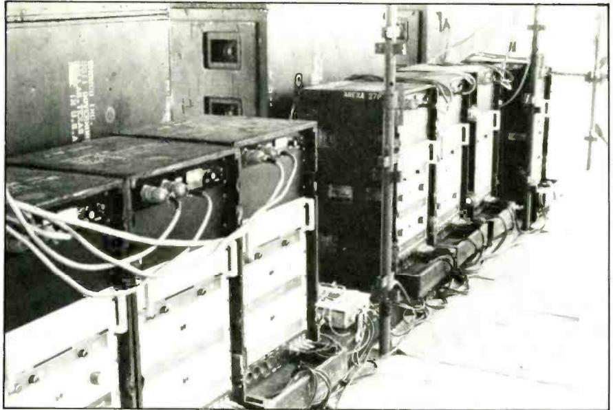
Figure 8: Showco amp racks for the delay towers: Crown DC-300-A and PSA-2 units, eight racks per tower.
