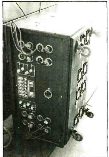
Figure 18: Clair's "Boat Anchor" amp rack: four 1,000-watt power amps in a compact box on wheels, complete with crossover and cooling fans for use with sidefill stacks.
