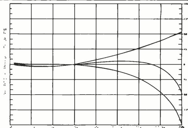
Figure 9: Relative Phase response. Bottom curve: model filter; top: optimized all-pass filter; center: corrected system.
