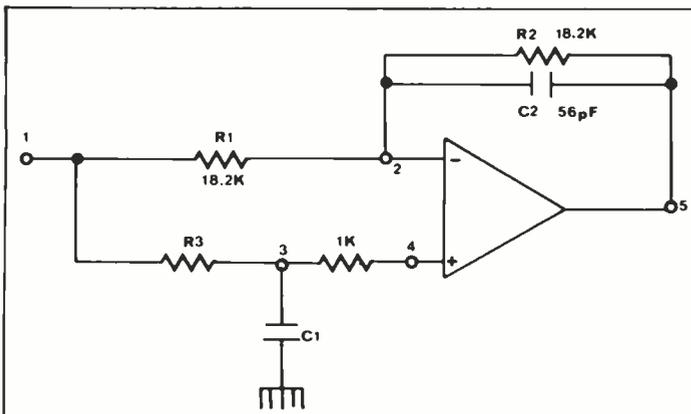
Figure 8: single-pole, all-pass filter configuration.
