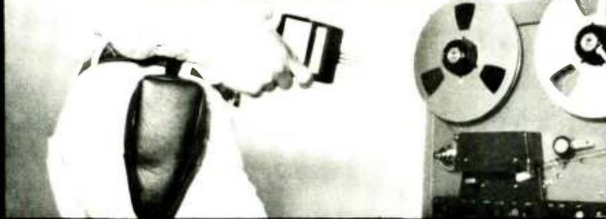
**The TENTELOMETER® in-line dynamic tape tension gauge is the fastest, easiest, most accurate method of diagnosing potential and existing problems in recording tape transports.**
