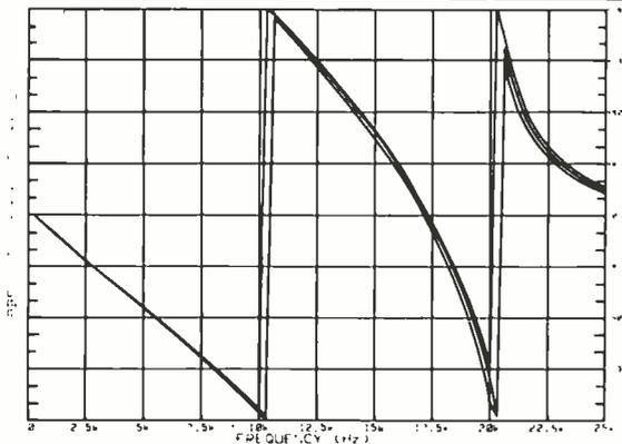
Figure 6: Absolute Phase response of optimized filter after 24 iterations; ±2% component tolerance limits.
