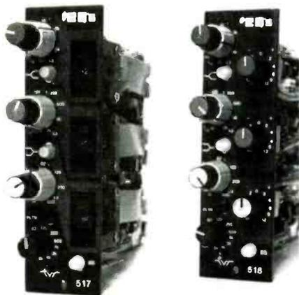
EQ range is adjustable from infinite cut to 15 dB boost (Model 517 has 12 dB max boost) with center-off positions that remove the filter circuits from the internal signal path. A fourth-band, second-order filter is included to selectively remove unwanted portions of the audio spectrum. A continuously variable frequency control covers the nine octave range from 31 Hz to 16 kHz for either low-pass, high-pass or notch filter modes.
