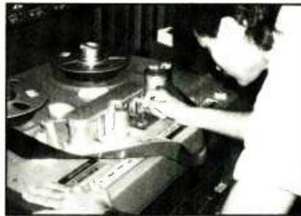
**Routine maintenance tasks that a second engineer can perform include keeping the multitrack heads and tape path free from dust and oxide residues.**
