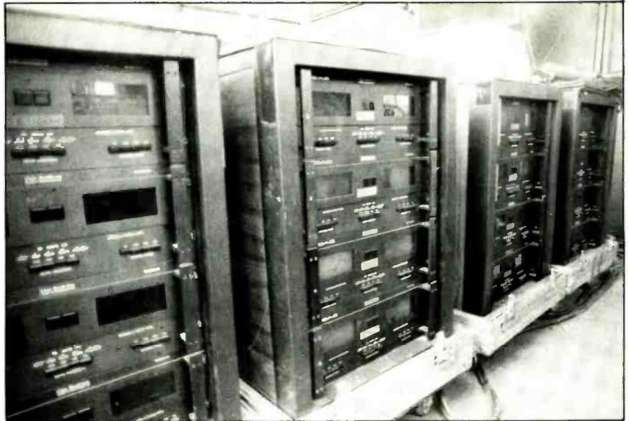
Figure 15: Racks of SAE 2600 amps, specially modified by Clair, to power the bi-amplified monitor mixes.
