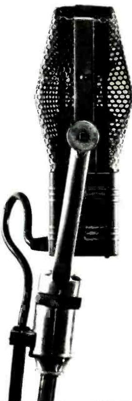
Coles 4038, the ribbon microphone par excellence of the BBC, is now available exclusively through Audio Engineering Associates. The Coles 4038 produces that warm ribbon sound without sacrificing highs. It features high output, low self-noise, excellent hum shielding, smooth frequency response, and uniform polar patterns.
