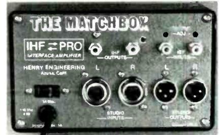
Two amplifiers convert a stereo high-impedance, unbalanced source to low-impedance, balanced outputs at studio operating level. A second pair of amplifiers converts a stereo balanced studio
