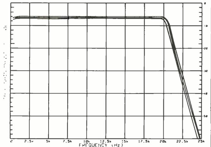
Figure 4A: Starting Model for filter magnitude response.
