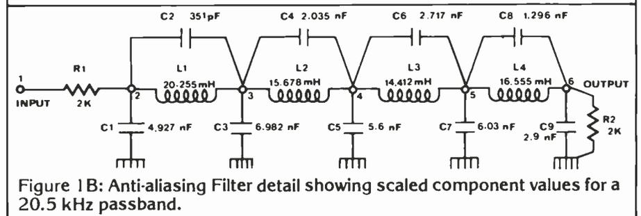
Figure 1B: Anti-aliasing Filter detail showing scaled component values for a 20.5 kHz passband.
