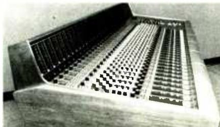
A dual metering system enables simultaneous display of both input signal
