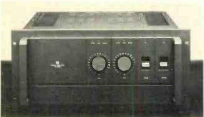
In addition, green and red LEDs are provided on each amplifier's front panel for quick visual confirmation of signal presence, circuit protect/thermal warning, and output clipping.
