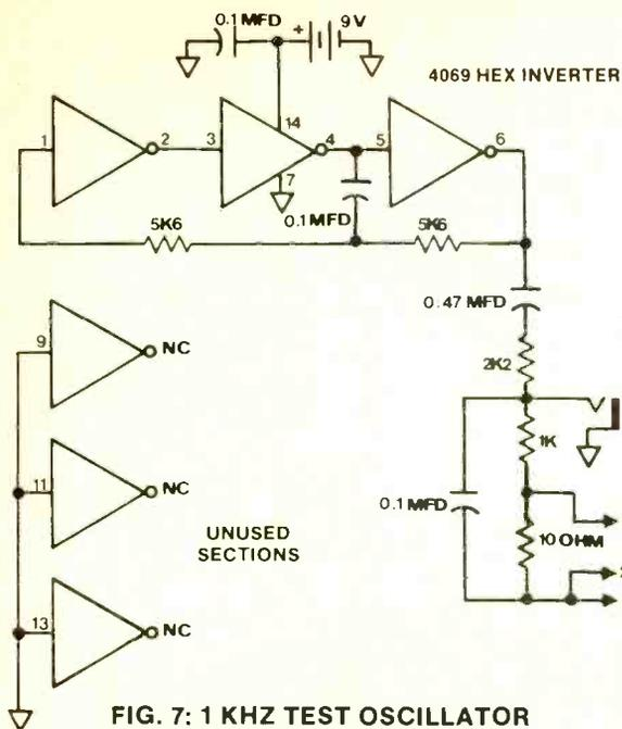
FIG. 7: 1 KHZ TEST OSCILLATOR
