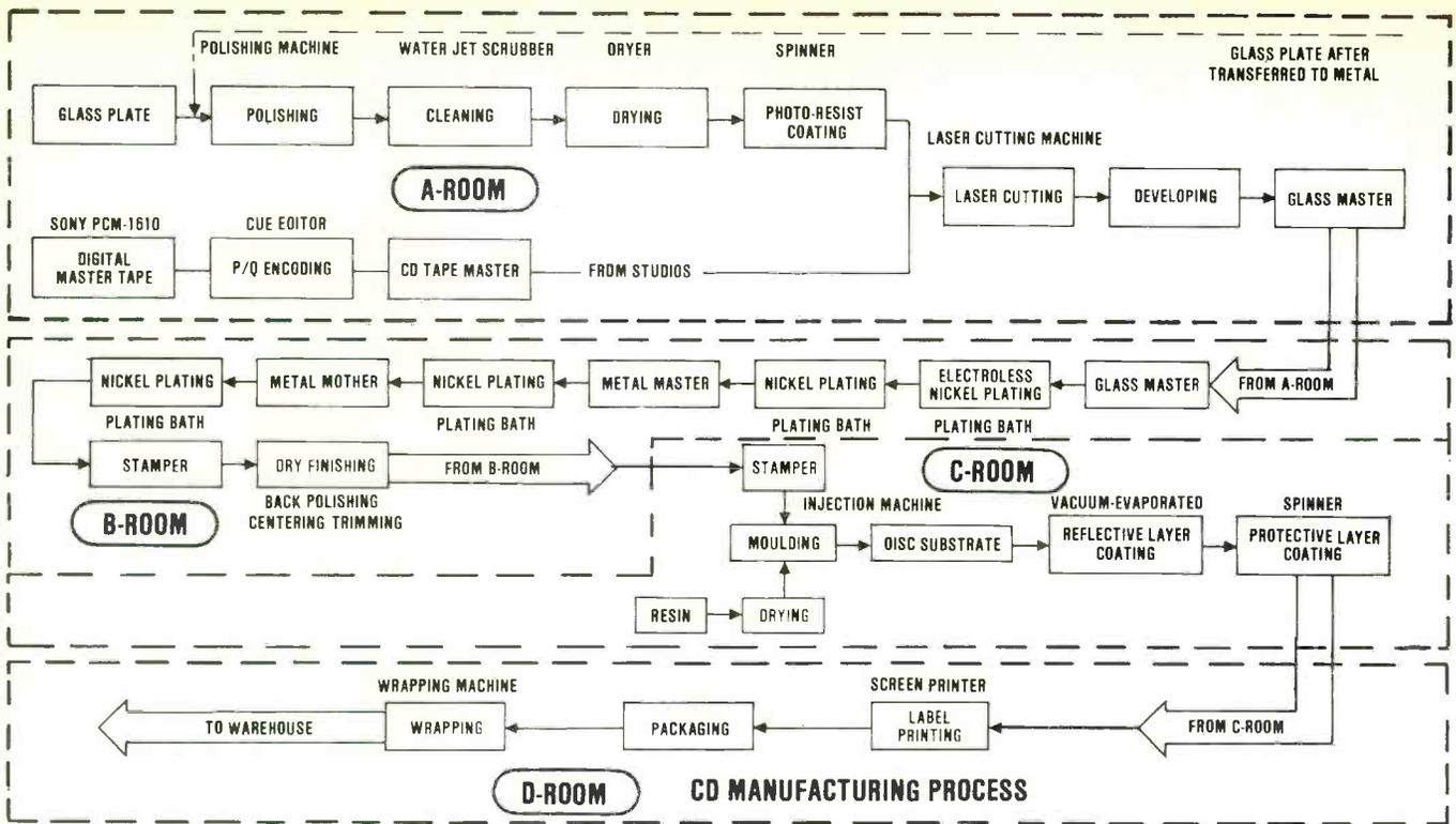
pickup system. Cycle time in the evaporator unit is 15 minutes. From here the CDs are placed on a continuous-feed unit that coats the lower surface with a protective layer, spins each Compact Disc to ensure complete coverage, and then utilizes an ultra-violet lamp to stabilize the coating.
