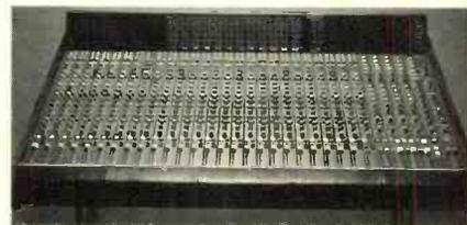
The Matchless comes standard in a 26/24 mainframe configuration, with larger frames and retrofit extenders also available. An optional version containing a full patchbay and producer's desk is forthcoming.
