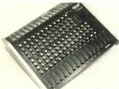
Professional-standard 48-volt phantom power also is included, plus three-band EQ on each input channel. Separate insertion jacks are provided for patching external effects into individual channels.
