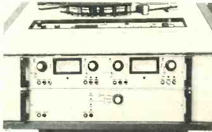
The JH-110-3-TC is available unmounted for standard 19-inch rack installation, or in variable profile (VP) or high profile (HP) cabinets.
