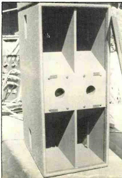
bass-horn technology apparently being used to an advantage to give the system a high perceived loudness factor with a minimum of loudspeaker cone area.
