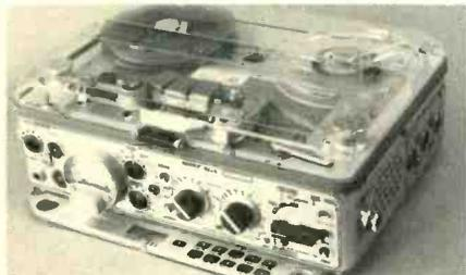
Mechanically the new machine is identical to the IV-S, the only difference being a thin sliding panel mounted underneath. The panel contains an LCD display and a mini keyboard used to read or enter data, and to check the operation of the system.
