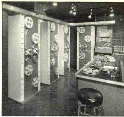
RCA mag dual dubber/recorders, MCI 24-track, & BTX Shadow synchronizers at MRI.
