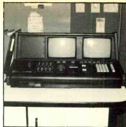
Strand Century Mini-Light Palette unit, which receives lighting control impulses from Allen Bradley PLC 2-30 computer.
