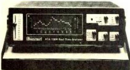
Both models are 27-band third-octave analyzers with frequencies set to standard ISO centers. A broad-band sound pressure level display is also provided, and consists of a matrix of 196 LEDs with selection of 1 dB or 3 dB per display step.
