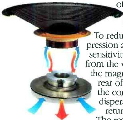
To reduce power compression and gain overall sensitivity, JBL created vents from the voice coil, through the magnet structure, to the rear of the loudspeaker. As the cone travels, heat is dispersed and cool air returned to the voice coil.
