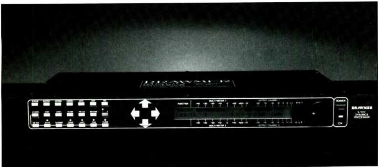
The M500 is a hybrid of technologies that brings dynamics processing into the digital age without sacrificing the advantages, real and perceived, of analog circuitry. It uses high-quality VCAs under digital control, and that control extends to the outside world through MIDI. The programmability of the unit is exceptional, and the user interface lets the engineer think about dynamics control in a musical context, greatly enhancing its creative potential.
