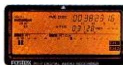
*The back-lit LCD shows all function data, including internally generated SMPTE timecode and A-Time, plus levels, program number, battery condition and error indications.*
