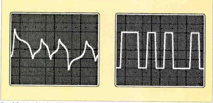
Figure 3. Depiction of waveform displays showing reshaping capabilities of SR-15 on original signals off analog tape (left) and end result (right).
