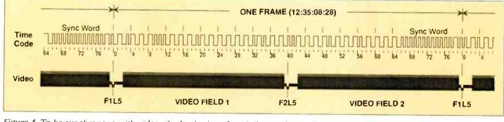
Figure 4. To be synchronous with video, the beginning of each time code word must coincide exactly with the beginning of the video frame it describes (i.e. time code bit 79 lines up with video Field 1, Line 5).
