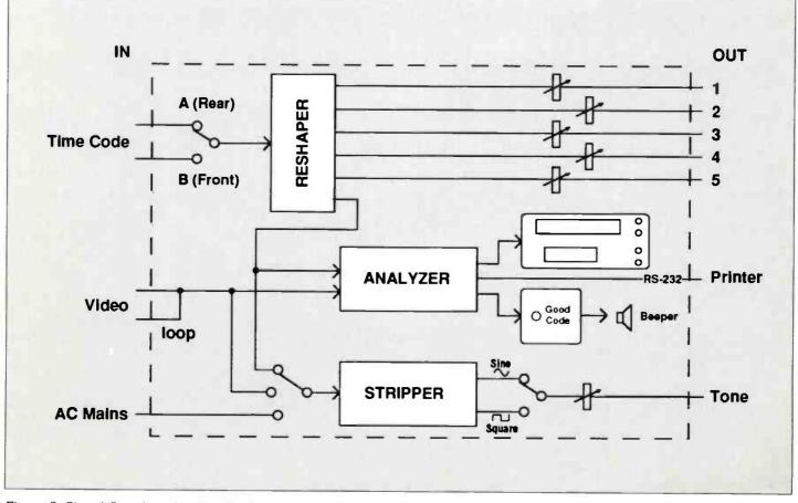
Figure 2. Signal flowchart for the SR-15 showing the reshaping, analyzing and stripper functions.
