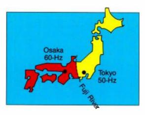
ing Tokyo are served by the Tokyo Power and Light Company with 60Hz service. Meanwhile, the western half of the country is served with 50Hz ac by the Osaka Power and Light Company. It seems that in the late 1890s each company imported generators (a 50Hz from Telefunken and a 60Hz from General Electric)
