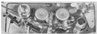
Fig. 3: View of the sound channel of the Wearite deck, snowing (l. to r.) automatic stop; erase and record/playback heads each with pressure pad; drive capstan and pressure roller (disengaged).
