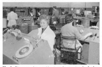
Fig. 5—The re-spooling machine (seen in operation in the foreground of the illustration) provides automatic inspection of the coating by a photo-electric system. In the background can be seen the machines for "pen-testing" Emitape.
