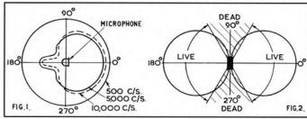
Fig. 1 Showing the tendency with most microphones for high frequencies to be lost, except for sounds arriving on the axis. Fig. 2 Figure-of-eight response of bi-directional ribbon microphones. Speakers or musicians placed in the "dead" angles are much reduced in volume.
