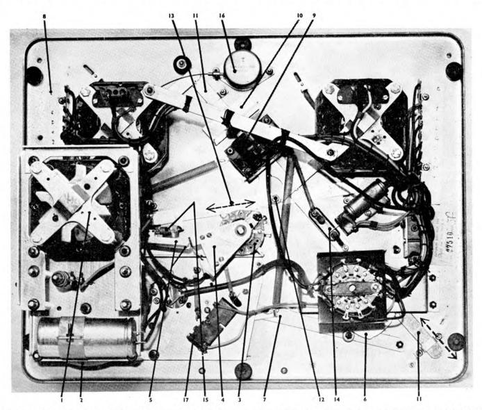
Fig. 4: 1. Drive motor 2. Fly-wheel 3. Wafer switch 4. Speed change plate 5. Push-links for 2 speeds 6. Cam plate for function control 7. Link 8. Tag panel 9. Electro-magnet 10. Contact for solenoid 11. Solenoid-operated link 12. Roller bearing 13. Link for braking 14. Power switch 15. Springs to idler wheels 16. Position indicator 17. Micro-switch.
