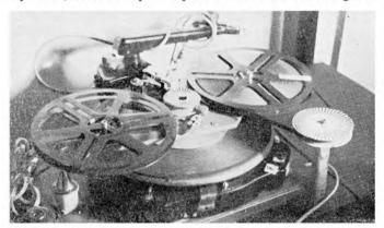
The writer of this letter enclosed the above photograph which illustrates the use of a Gramdeck unit and an old-fashioned gramophone. The sound track can be set to keep in sync. with a fixed speed projector. The stroboscope is driven by the tape and lit by the projector flicker.
