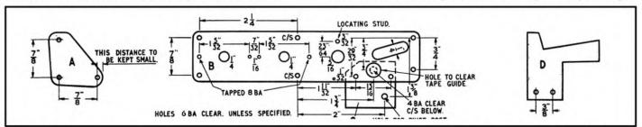
Fig. 2. The four metal plates. Plate A is bolted to the tape tension arm. Plate B replaces the existing head mounting strip, with Plate C fitted underneath to take the extra pressure pad. Plate D holds the Record and Erase pressure pads clear of the heads, except when recording.
