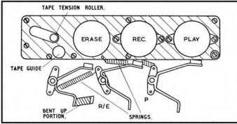
Fig. 1. Showing the relative positions of the extra head and the Erase, and Record/Playback heads on the Plate B. This drawing is to scale relative to the large photograph in the Collaro Instruction Manual, and an accurate picture of the placement may be got by tracing this diagram and laying the tracing over the photograph.
