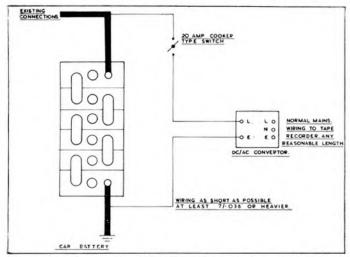
Fig. 1. Showing the connections from the car battery to the DC/AC Convertor. It is important to keep this wiring as short as possible, and to use heavy gauge cable.
