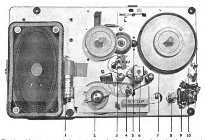
Top view with cover removed, showing 1. electrolytic smoothing condenser, 2. selector switch, 3. idler wheel, 4. permanent magnet erase head, 5. drive capstan, 6. record/playback head, 7. rubber rim on tape-up spool to take drive and brakes, 8. recording level/volume control (knob removed), 9. motor control transistor, etc. 10. Brake arm for take-up spool.
