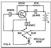
Fig. 4. Shows a method of using a double-pole, doublethrow switch to change over the transducer and the Record/Replay head for recording or playing back. This diagram is included for experimenters who are able to assemble more complicated arrangements helped by the circuit above.
