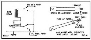
Fig. 3. (Left). Typical head switching circuit, showing the use of a humbucking coil. Fig. 4. (Right). A thin dural mount as shown allows the coil to be tried in different positions for best effect.
