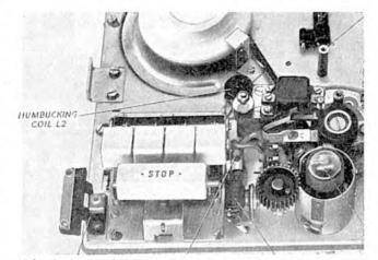
A humbucking coil is featured in a number of tape recorders. The photograph shows the early Grundig 500L/700L series machine.
