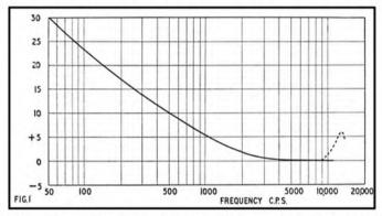
of gap loss and head loss (far from ideal) the playback response will be modified as in the dotted line, and this variation will be individual to the particular machine, or, rather, the playback head.
