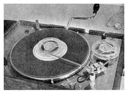
turn up an aluminium or brass adaptor. A heavy 4-in. brass disc would be most suitable as it would add inertia smoothing to the take-up and ensure a performance only slightly inferior to the more bulky turntable.
