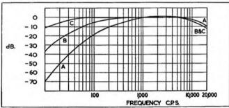
Fig. 1 Loudness meter curves for A below 55 dB, B 55 to 85 dB, C over 85 dB.
