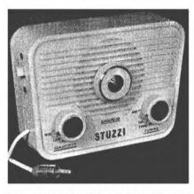
Yet, if your "domestic environment" is anything like mine, the chances are that the family tape enthusiast cannot always have access to the family radio set, and it is to get round this problem that the various tape tuner units and tape jacks have been manufactured. They consist of transistor receivers producing an audio output at a fraction of a volt or, in the simplest examples, of a crystal detector set pre-tuned to a single station.
