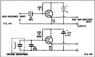
Fig. 4 Two possible circuit modifications for crystal microphones.
