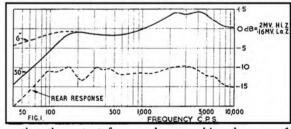
shows that the output for sound approaching the rear of the microphone is down 10 to 12dB over most of the frequency range. This is because the phase change in the acoustic resistance
