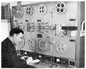
Mr. Hanks, the head of the recording department, at the transfer machine where 16 mm magnetic tracks are prepared, for subsequent mixing. The nearest panel carries a sound-on-film camera which makes the optical track needed for release prints.
