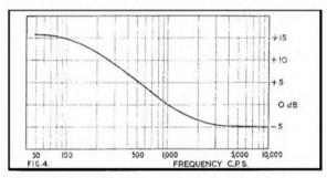
seconds for 3½ i/s. This at least has the merit of lining up with the 15 i/s 35 microsecond standard so that, theoretically anyway, the same test tape could be used at all speeds, and the frequencies halved or doubled according to the speed.
