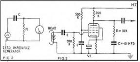
made the exact inverse of the recording characteristic by using the same time constant in a different circuit configuration.
