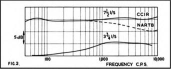
Fig. 2. Replay only response 100 and 200 µsec Test Tapes
