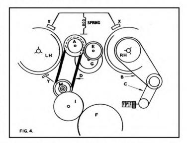
As a further note on Grundig belts, we should perhaps deal briefly with some aspects of the TK14. (It is hoped to go into greater detail on this popular machine at a later date.) At present, we are concerned mainly with the query received from some readers about the adjustment of the motor pulley and the fitting of a different belt.
