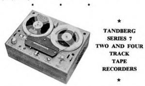
THE introduction of the Tandberg Series 7 has been announced by the distributors in this by the distributors in this country, Elstone Electronics Ltd. Two versions are available, the Model 72 (two track) and Model 74 (four track). Three speeds are provided, 7½, 3¼ and 17 i/s. The claimed frequency response is 30-20,000 c/s at  $7\frac{1}{2}$  i/s; 30 to 14,000 c/s at  $3\frac{1}{4}$  i/s; and 50 to 7,000 c/s at  $1\frac{1}{4}$  i/s. Wow and flutter figures quoted are within 0.15%; 0.2% and
