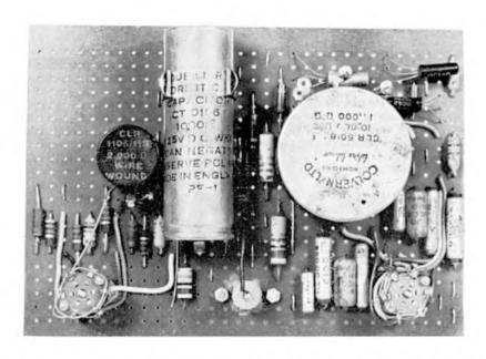
tance), of the circuit shall be long enough to pass the low frequencies without attenuation. In a valve oscillator most circuits would be high impedance, capacitors are correspondingly small, and a cathode follower stage has to be added in order to have the low output impedance that is necessary. With transistors the circuit impedances are already relatively low, and so it is simpler to increase the capacitor value rather than add what would here have to be an emitter follower.
