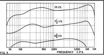
at  $3\frac{1}{4}$  i/s confirms that the bias was indeed about right for the tape speeds provided by this deck—a little high for  $3\frac{1}{4}$  i/s—2 little low for 15 i/s—and just right for  $7\frac{1}{2}$  i/s. For a lower speed deck 40 volts bias would probably be all right. The response on the lower track was next tested and found to be almost identical to that of the upper track.
