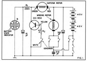
in fig. 1. Note the two 4.5 volt batteries in series, supplying the motors with 9 volts. The amplifier has a separate power
