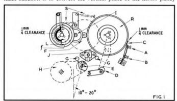
axis to the horizontal plane for the belt to wrap the flywheel groove. Note that there have been three different types of motor supplied, and the connections vary. The original motor was nickel-plated, had yellow and white switch leads and red and green motor leads. Its replacement, known as Type A, had yellow and black switch leads, and the motor leads were either red and green or red and blue, according to the production run.
