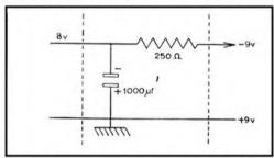
whatsoever. If a higher voltage supply is available, the resistor can be increased in value to advantage. Or for that matter the capacity of the electrolytic can also be increased.
