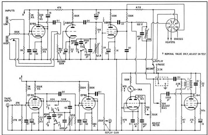
Fig. 1A: Circuit diagram and component values for use with the Planet U1 tape deck. Since passing this for press the author has sent in the following alterations: 220 Kohm resistor should be placed between the anode of the first half of the 6BRB valve and 0.1 \( \mu f \) capacitor. The 30K bias adjuster open side should be taken to chassis.
