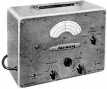
An Audio Signal Generator may be a beat frequency oscillator or a resistance / capacitance phase shift oscillator. The B.F.O. offers the considerable advantage of covering the whole audio range in one sweep, but the phase shift type is generally more accurate for a limited outlay.
