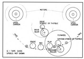
Fig. 3: Main parts of a conventional three motor tape deck showing, erase, recording and playback heads, capstan, pressure roller, flywheel, drive idler, and drive spindle or thimble.
