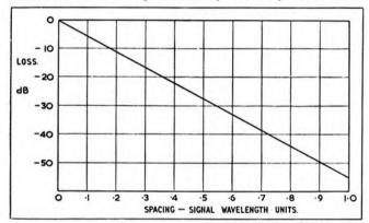
Fig. 2: Effect of Head-Tape separation. The horizontal scale can be read directly (full-scale=1 thousandth of an inch) for a signal wavelength of 1 thou', e.g. 7.5 Kc/s at 7½ i/s, 3.75 Kc/s at 3½ i/s, 1.875 Kc/s at 1½ i/s, etc.; or with full-scale of half this for twice these frequencies and similarly for other wavelengths in inverse proportion.
