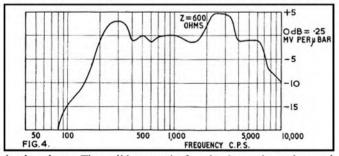
loudspeakers. The solid curve is for the internal speaker and the dotted curve is for the external lid speaker. These responses were taken at a tape speed of  $7\frac{1}{2}$  i/s so as to measure mainly the response of the speakers and enclosures.
