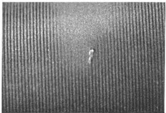
Fig. 4: Two more nodules on old, stiff tape. Magnification x 40.
