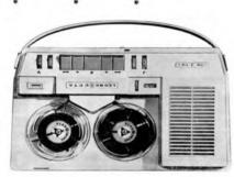
Manufacturer's Specification. Power supply: A.C. 40-60 c/s 110-220 v, 6 v car battery, 12 v using series resistance LR412, 5 U2 torch cells, 5 DEAC rechargeable cells type RS3.5. Recording procedure: double track international standard. Tape speed: 3½ i/s. Frequency response at radio output: 50-10,000 c/s. Dynamic range: 46 dB or better. Maximum reel diameter: 4½ in.
