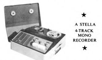
The machine is supplied with a five inch spool of long play tape, but the deck has been designed to take seven inch reels. By using an additional pre-amplifier, together with an amplifier and loudspeaker pre-recorded stereo tapes  $(3\frac{3}{4} i/s)$  can be played. A parallel playback facility enables simultaneous replay of tracks one and three or two and four.
