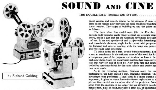
The Siemens 800 projector showing the double-band attachment side with sprocket and four film guides. The magnetic heads are contained in the lower housing which is hinged, allowing free access to the heads for marking up. Both picture and sound spools are fitted with easy-loading device.
