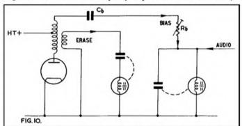
Fig. 10. Typical resonant feed circuits for low-impendance erase head and high-impedance record head. Resonant combinations shown by dotted lines; erase in series, record in parallel.
