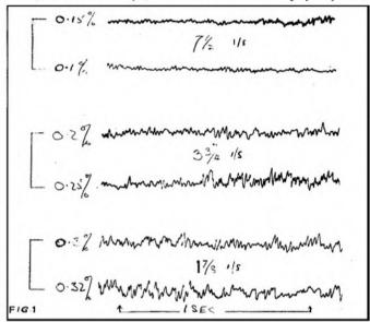
At no time was there any suspicion of speed unsteadiness. A sustained musical note sounded dead on pitch although there was this constant feeling of slight roughness. I can usually recognise the effects of under-biassing, overmodulation or various types of tape flutter, but this was different, and I proceeded with my measurements with some interest to try and uncover the exact cause of the trouble.
