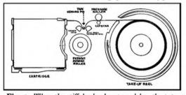
Fig. 2. When the stiff leader has passed by, the tape sensing pin drops down to engage the tape with the heads; the feedout drive roller is disengaged and the pressure roller and capstan come together.
