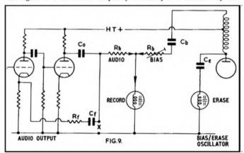
Fig. 9. Possible DC leakage paths, causing high background noise on tape, through Co, Cf, Cb, and Ce.
