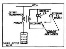
Fig. 1. This diagram shows how a switched jack socket can be wired to the loud-speaker circuit so that when the plug carrying the external speaker is inserted the internal speaker is automatically switched out of circuit.
