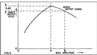
Fig. 3. The optimum bias setting taking into account signal-to-noise ratio and distortion should be determined aurally. The best setting will normally be found somewhere between A and B; i.e. a slightly higher bias level than that giving maximum recorded signal level.
