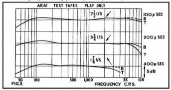
the bias field penetrates to the full depth of the oxide, but the bias field dies away gradually on either side of the gap so that oxide particles, properly magnetised within the gap, are partly erased as they pass through this diminishing field so that short wavelengths, comparable to the dimensions of the fringing flux, are most affected leading to a lack of high note response which has to be made good by extra high frequency pre-emphasis in the recording process. See fig. 1A.
