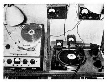
The cutter is moved in to the correct starting diameter and the tape started whilst the volume is increased to required level, this having been decided during the test cuts. All is safe now and a matter of close watch on the special volume indicators connected to the cutter-head, to avoid any sudden bursts that would force the stylus over, causing both distortion and cutting through into next groove.
