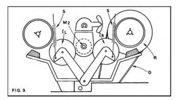
is simply pressed into rubber grommets. It is necessary to hold back the pressure pads with the fingers when removing and replacing the arm, and to ensure that the tension spring at the right-hand end is properly located after re-assembly.
