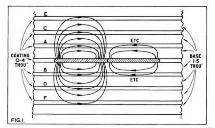
This shows adjacent layers of tape on a spool with two half-wavelengths of master signal (recorded 500 c/s at T½ i/s) to scale, and flux lines passing through other layers, not necessarily to scale.
