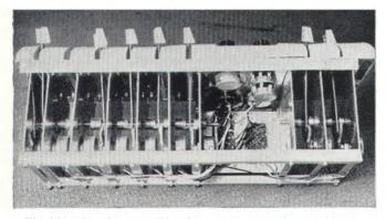
Fig. 2(a): Complete assembly of potentiometers with control levers.
