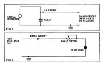
woolly, and the speech too harsh. Some compensation for the harsh speech quality can, however, be taken. A simple top-cut circuit could be incorporated as shown in fig. 3, and adjusted by trial and error until the best setting is found.
