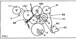
Model 101. This is a machine with a four-transistor pre-amplifier circuit driving a 6AR5 valve output, doubling as HF oscillator for recording purposes, with a 5MK9 valve rectifier. The spool and flywheel drive is via four separate idlers, with a single function selector lever and spring return action throughout. Fig. 1 gives some indication of the mechanical system and notes the clearances to be obtained from the following adjustments.
