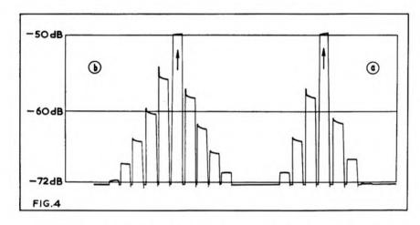
This and fig. 2 shows a print series on (a) Standard Play tape, (b) Long Play, and (c) Double Play. Preprints are to left of master-signal (marked with an arrow).
