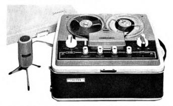
Full facilities for 1-track recording and replay, as well as MULTIPLAY and inter-track recording, are offered by the CR1607 (shown with microphone), with speeds of 32 and 12 i/s. Peak-to-peak wow and flutter figures of 0.6% are claimed, with a frequency response from 80 c/s to 15Kc/s at the faster speed and 80c/s to 10Kc/s at 17 i/s.
