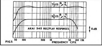
Hum and noise was 40dB below test-tape level at  $7\frac{1}{2}$  i/s and 35dB below test tape level at  $3\frac{1}{2}$  i/s. Later recording tests showed that a level 12dB above test tape level could be recorded without distortion at either speed, so that the effective signal noise ratio is 52dB at the higher speed and 47dB at the lower speed.
