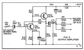
expensive silence! The voltages on the circuit diagrams can be checked against the values actually obtained. For this, any instrument will be satisfactory since the circuits are low impedance and will not be unduly loaded.
