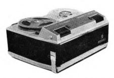
**F**OUR new recorders have been added to the *Grundig* range—Models *Luxus TK* 14*L*, *TK* 17*L*, *TK* 18*L* and *TK* 23*L*. Common specificational points are tape speed -  $3\frac{1}{4}$ i/s; frequency response - 40 c/s to 12 Kc/s  $\pm 4$ dB; wow and flutter -  $\pm 0.2$ %; output power - 2.5W; dimensions -  $13\frac{1}{4} \times 10\frac{1}{2} \times 6\frac{3}{4}$ in.; weight - 22lb. All four incorporate high impedance and external speaker outlets and all are mains powered.
