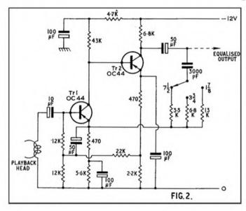
AST month we saw the need for playback equalisation. We saw that the EMF induced into the playback head winding rises constantly at 6dB per octave up to the turnover frequency, at which point the EMF commences to drop slowly at first and then fairly rapidly. Previous articles in this series have shown why this happens.
