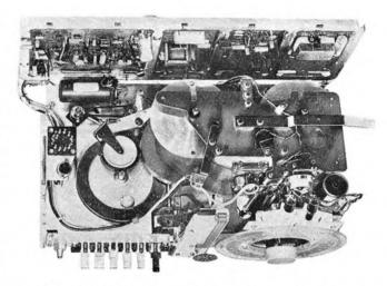
operates on 126 tracks, each with a twenty-two minute playing time on 4in. tape. Two models are available, one with built-in radio and the other with radio and disc-player. The twenty-two minute single-track playing time was selected to correspond with that of an LP disc and to record from disc or radio it is necessary only to press a single button.
