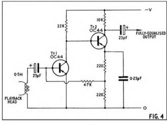
end of the spectrum, since the filter would cause a progressive reduction in signal from the head to the amplifier from the bass end up to the turnover frequency. Moreover, the insertion loss of the filter would reduce the nominal signal applied to the input of the amplifier from the head.
