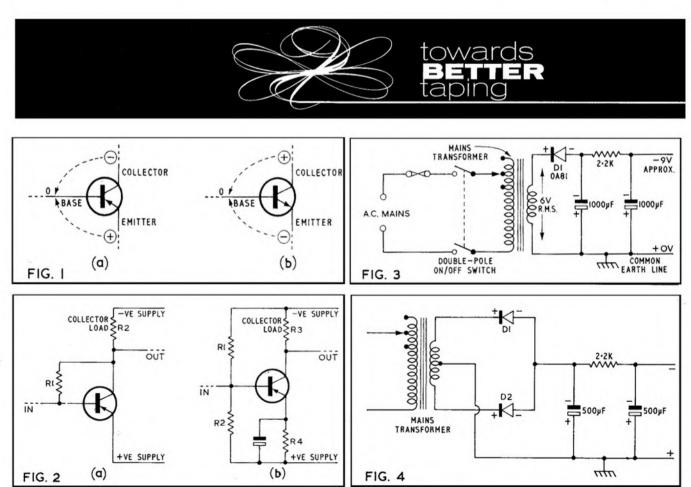
Alternatively, a small mains power unit can be constructed solely for powering the transistor amplifier.
