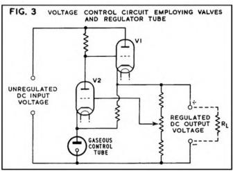
voltage stabilised by the gaseous control tube with respect to the negative line, the cathode being held at a constant positive voltage with respect to the grid. This means that the fall in output voltage—making the grid go less positive—will increase the negative bias on the valve, thereby decreasing the anode current of V2 and causing a rise in anode voltage.
