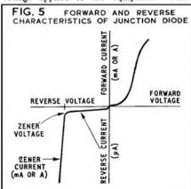
larly, if the input voltage dropped to 12V, the zener current would fall proportionally, reducing the volts drop across Rs and again holding the equipment voltage constant.
