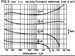
speed of 15/16 i/s, as there was under-signal noise mixed up with the 3Kc/s test-tone which made measurement difficult.
