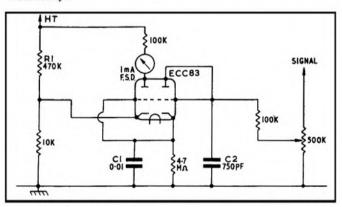
The circuit is straightforward. The 470K resistor R1 could be altered to give exact balance, and if you want a better delay characteristic (this is a peak-reading type) increase C1 to 0.015 or 0.02mF. The capacitor C2 is important, being 750 pF and preferably a good disc ceramic, as this one performs the function of by-passing the bias from the detector.
