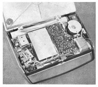
Optacord 416 with lower lid removed. Battery storage tube and mains lead are visible at rear, motor housing being seen at lower left.
