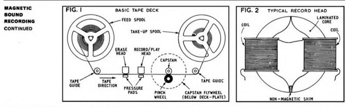
head for both recording and reproduction and a second head for erasing. A section of a typical head is shown in fig. 2. It consists of a laminated coil of some such material as *Permalloy*. This has a very narrow hysteresis loop, which means that it can be magnetised with ease but loses its magnetism immediately the magnetising field is removed. Narrow gaps at each end of the core are filled by nonmagnetic 'shims' and on each side a multi-turned coil is wound.
