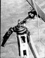
Above: Lightweight Hammond M.100 capacitor microphone on universal bracket and Terry Clip. Left: Swivelling pillar and ball joint of ex-army tripod. Below Left: Mk. I boom set up against a small Willis pipe organ. Below: Mk. II boom with
